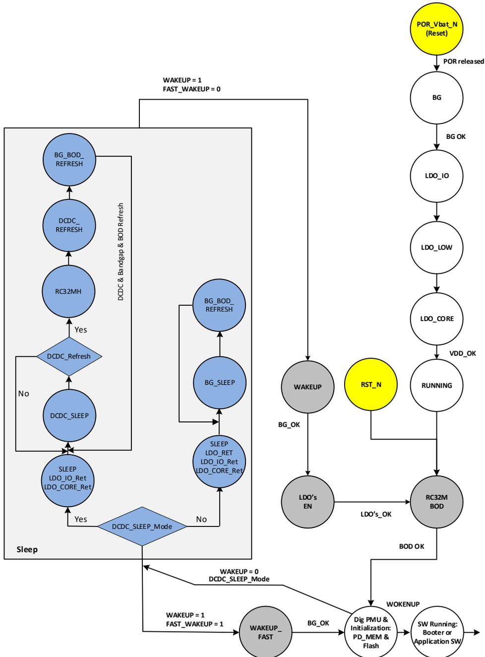
Figure 5. POWERUP, WAKEUP, GOTO SLEEP hardware FSM
