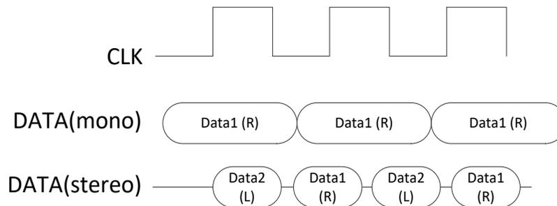
Figure 55. PDM mono/stereo formats
