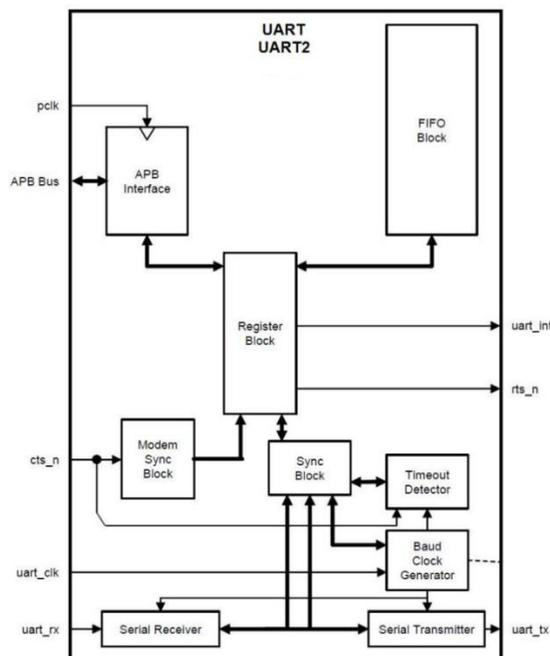
Figure 67. UART block diagram
