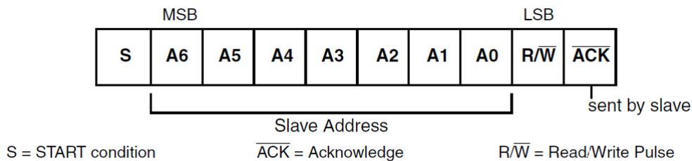
**Figure 60. 7-bit address format****10-bit Address Format**
