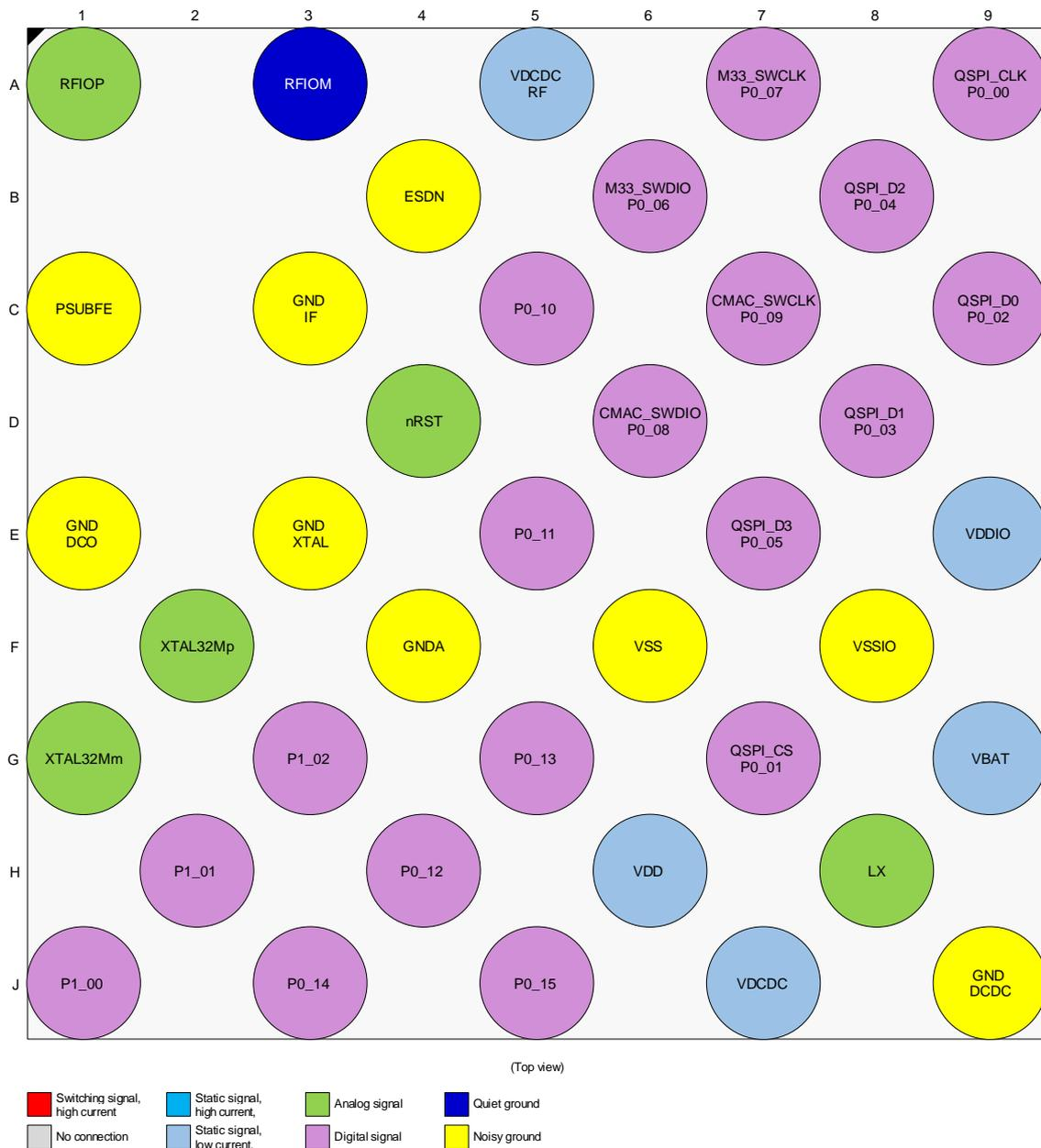
Figure 2. WLCSP39 ball assignment
