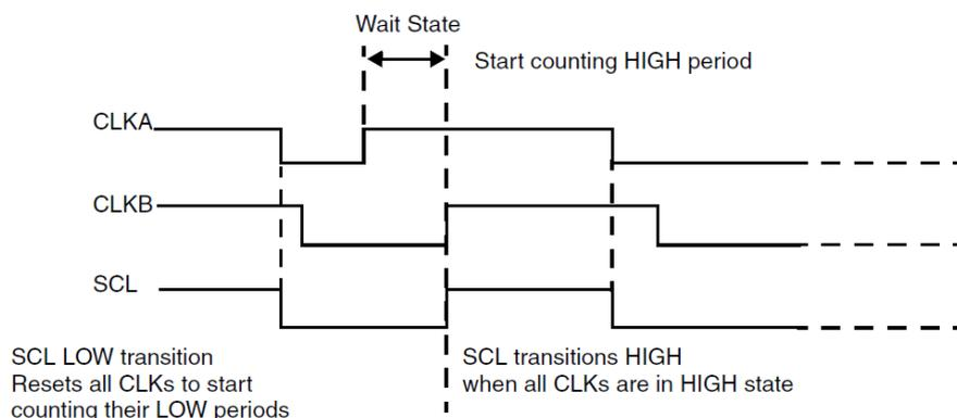
**Figure 66. Multiple master clock synchronization**
