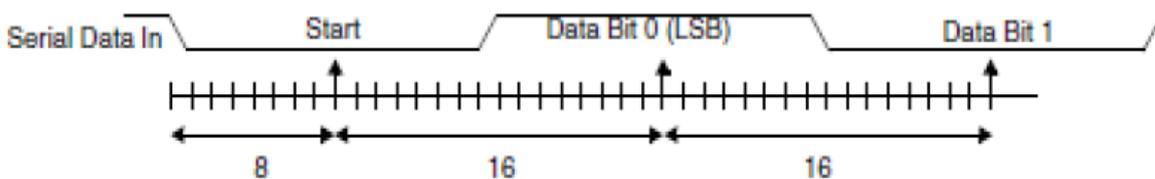
Figure 69. Receiver serial data sampling points
