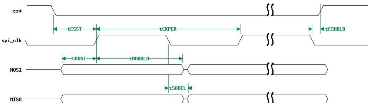
**Figure 74. SPI Slave mode timing (CPOL = 0, CPHA = 0)**
