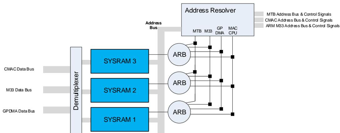
Figure 25. Internal architecture of the memory controller
