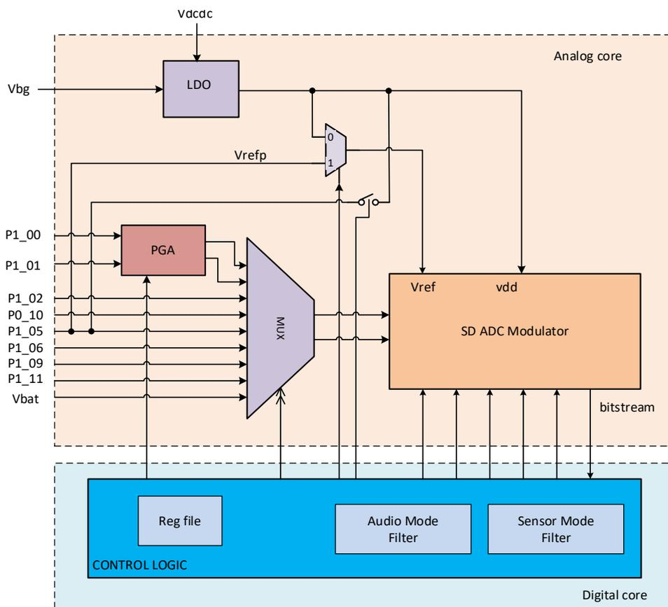
**Figure 44. Block diagram of the ΣΔ ADC**
