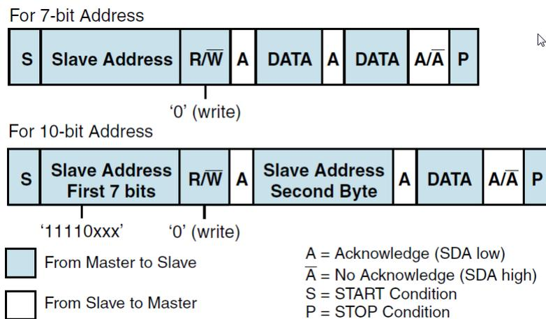
Figure 62. Master-transmitter protocol
