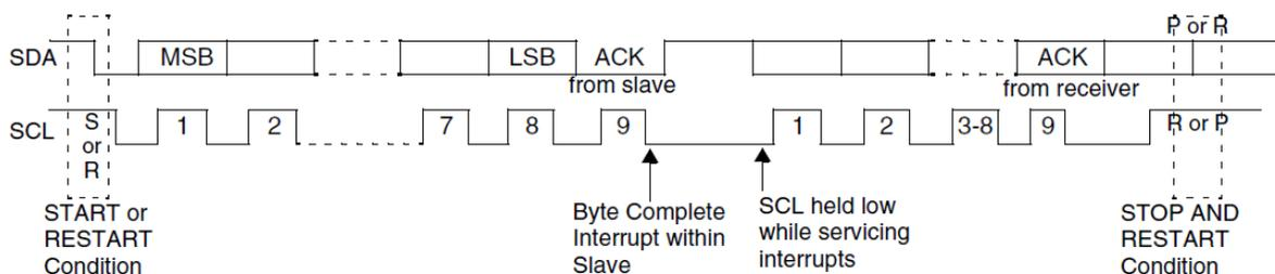
**Figure 58. Data transfer on the I2C bus**
