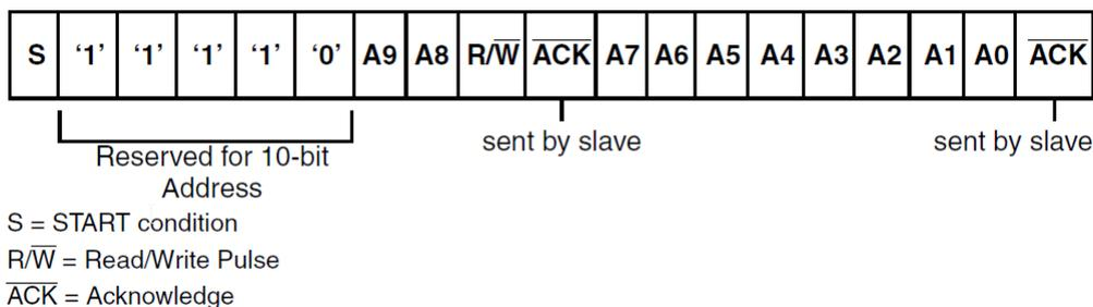
**Figure 61. 10-bit address format****Table 96: I2C Definition of Bits in First Byte**
