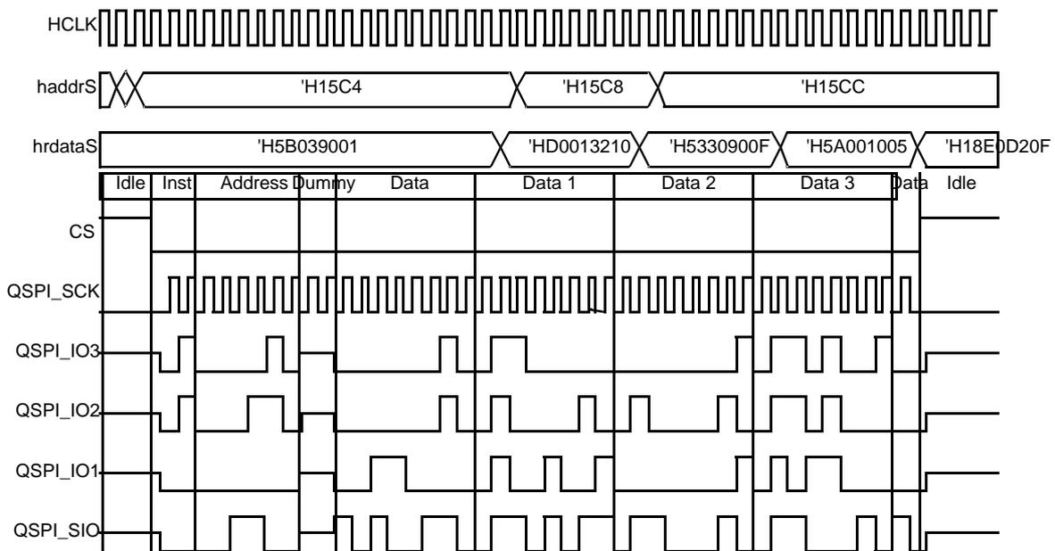
Figure 34. QSPI burst timing for high performance (QSPI\_FORENSEQ\_EN = 0)
