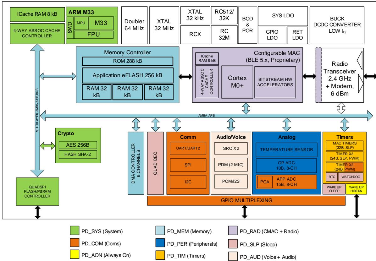
Figure 4. Digital power domains and blocks mapping
