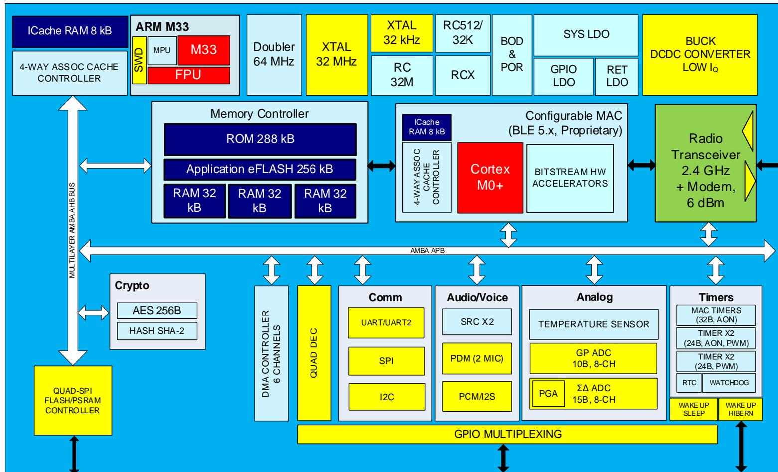
Figure 1. DA14592 block diagram
