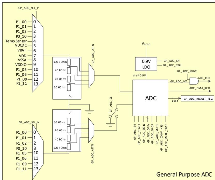
Figure 42. General-purpose ADC block diagram
