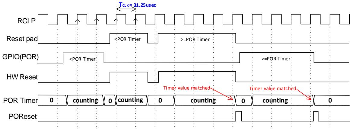
Figure 20. Power-on reset timing diagram
