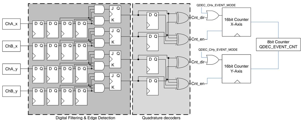
Figure 78. Digital filtering and edge detection circuit
