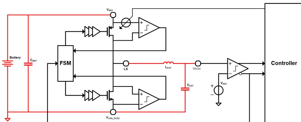
**Figure 15. DCDC converter block diagram**
