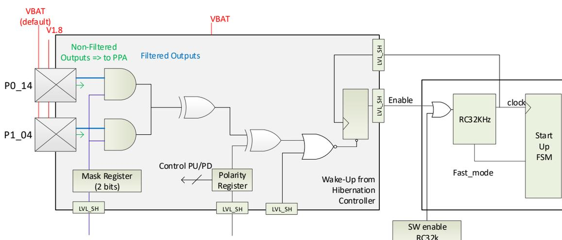
Figure 41. Wake-up from hibernation controller block diagram
