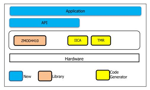
Figure 5.1 Software Structure
