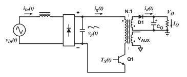
Figure 9.2: Simplified Flyback Converter
