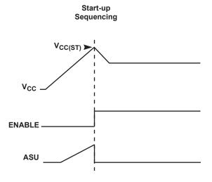
Figure 9.1: Start-up Sequencing Diagram
