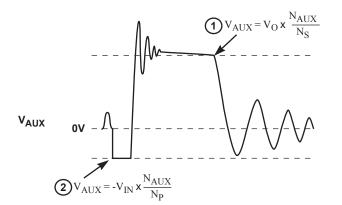
Figure 9.3: Auxiliary Voltage Waveforms
