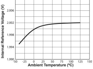
Figure 7.4 : Internal Reference vs. Temperature
