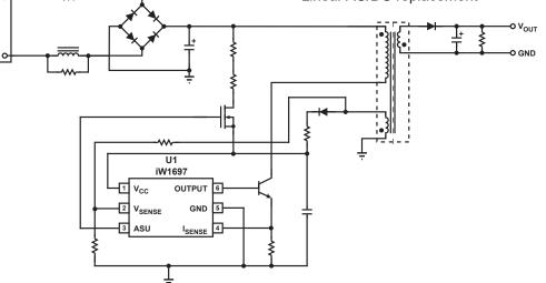
Figure 3.1: iW1697 Typical Application Circuit
