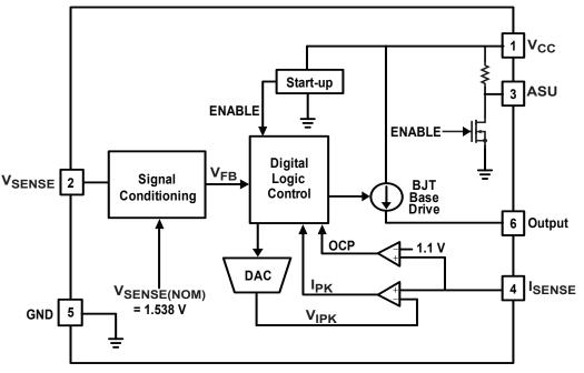
Figure 8.1: iW1697 Functional Block Diagram
