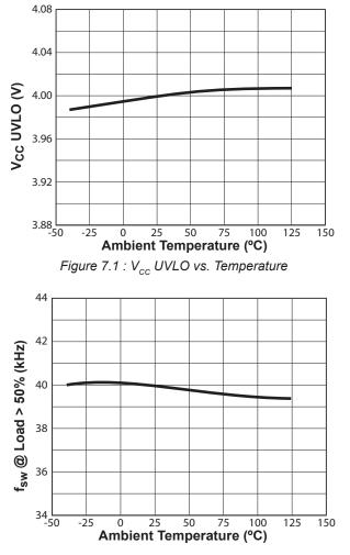
Figure 7.3 : Switching Frequency vs. Temperature<sup>1</sup>
