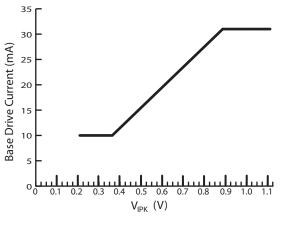
Figure 9.5: Base Drive Current vs. V<sub>IPK</sub>
