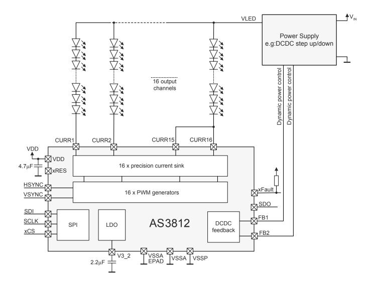
Figure 3.1 : AS3812 Typical Application (With CURR15 and CURR16 connected together to show increased LED string current capability by paralleling outputs)
