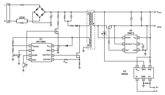
Figure 3.2 : iW1780H Typical Application Circuit for Multi-Level Output Voltage and Current (Using iW636 as Secondary-Side Controller for QC3.0 and iW673 as Synchronous Rectifier Controller Achieving < 20mW No-Load Power Consumption in Typical 15W Design)
