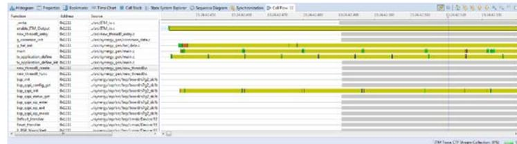
This feature enables PC sampling which then will return the PC location at a user defined interval. The program flow at each of these intervals is then graphed.
