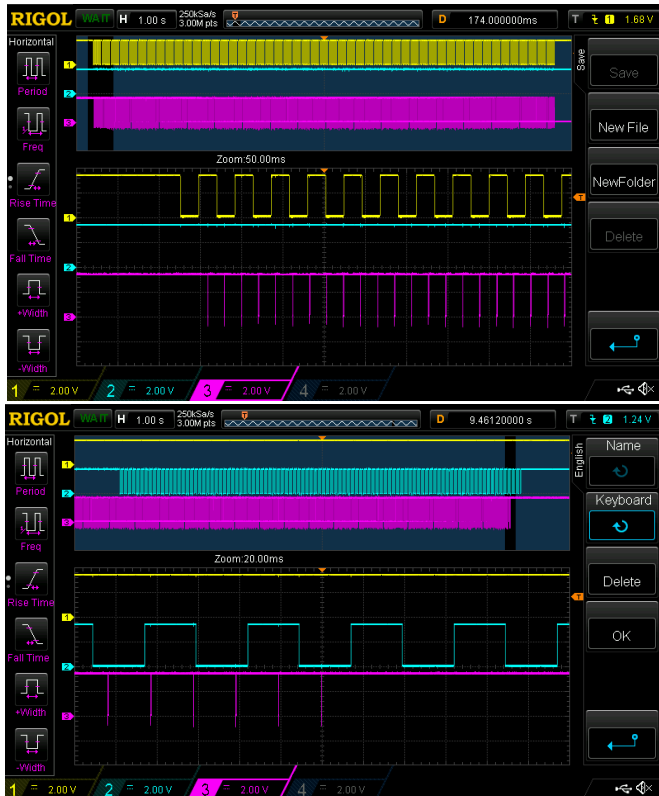
Figure 10. LED Brightness Control _3 waveforms. Top line is button “+” input, 2nd line is button “-” input, 3rd line – LED output
