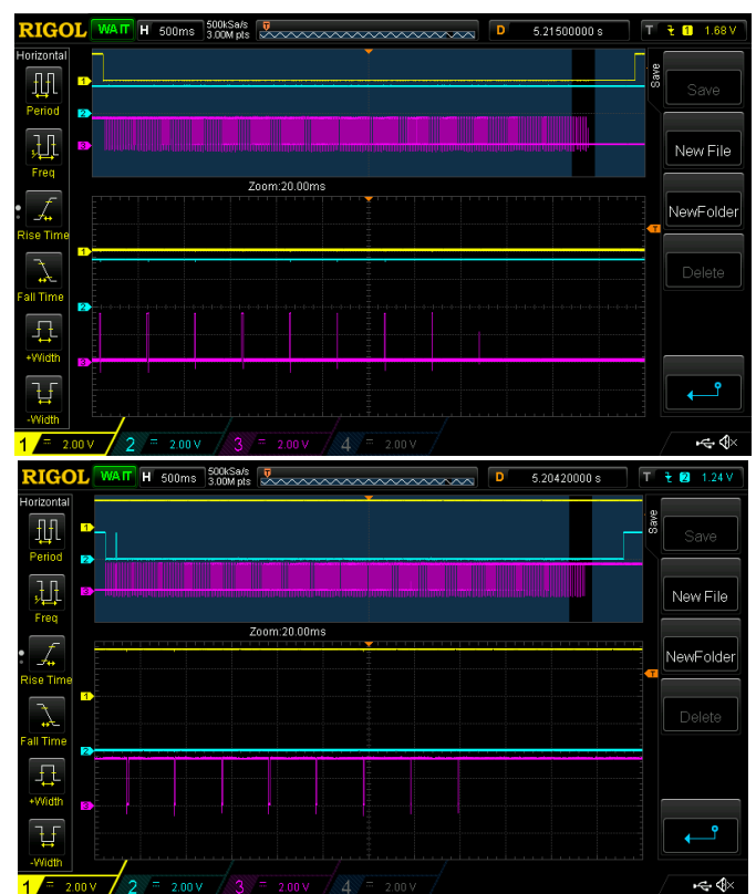
Figure 9. LED Brightness Control_2 waveforms. Top line is button “+” input, 2nd line is button “-” input, 3rd line – LED output
