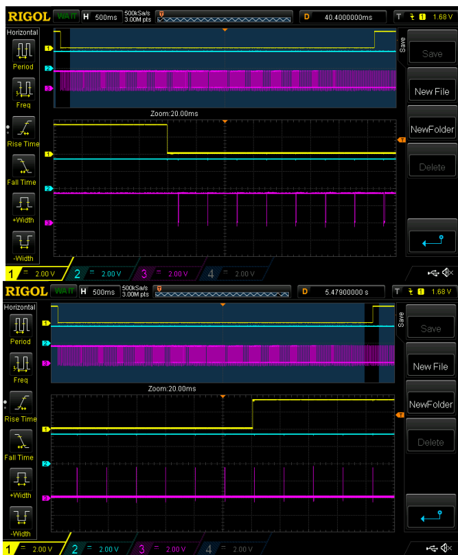
Figure 8. LED Brightness Control_1 waveforms. Top line is button “+” input, 2nd line is button “-” input, 3rd line – LED output
