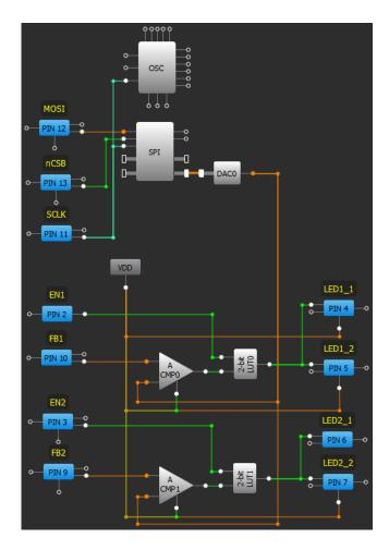
Figure 1. LED constant current circuit design
