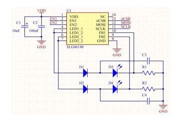
Figure 2. LED constant current typical application circuit
