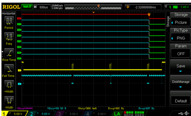
Figure 3. I2C Command [0x00, 0xF4, 0x00]
