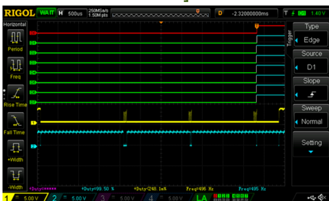
Figure 4. I2C Command [0x00, 0xF4, 0xFF]
