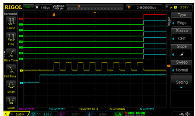
Figure 6. 1us scale of Data Byte 0xFF
