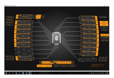
Figure 2(c). GreenPAK emulator window in Emulation Mode
