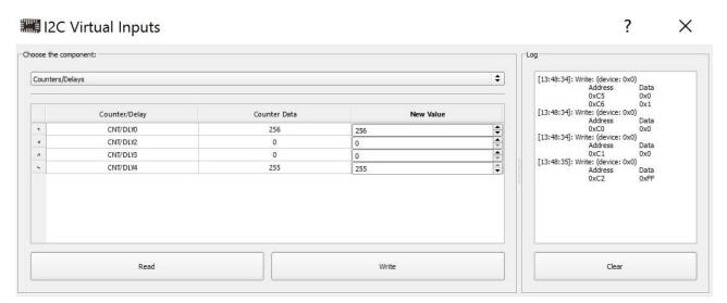
Figure 3(f). GreenPAK I2C Virtual Inputs for 100% PWM setting for blue LED
