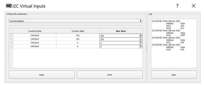
Figure 3(b). GreenPAK I2C Virtual Inputs for 100% PWM setting for red LED
