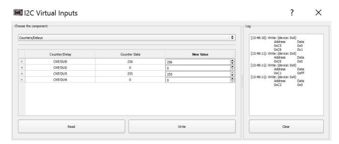
Figure 3(d). GreenPAK I2C Virtual Inputs for 100% PWM setting for green LED
