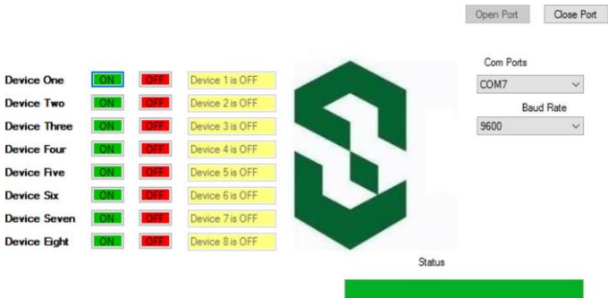
Figure 8. Visual C# Application for Receiving/Sending Data to/from consumer
