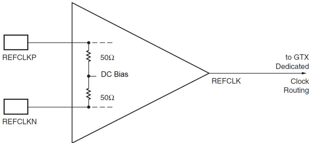
The reference clock input on the Xilinx FPGA has on-chip 100Ω (50Ω + 50Ω) differential termination. The center tab between the two 50Ω resistors is biased internally and Xilinx recommends to AC couple the differential reference clock with typical 100nF capacitors to the REFCLKP and REFCLKN input pair.
