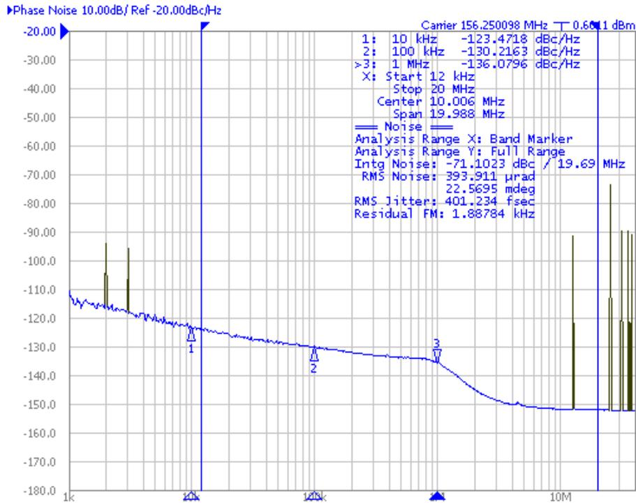
A few spurs appear above 30MHz but still no significant contribution to phase jitter or phase noise levels. This combination is perfect for the 5P49V6901 with four differential outputs.
