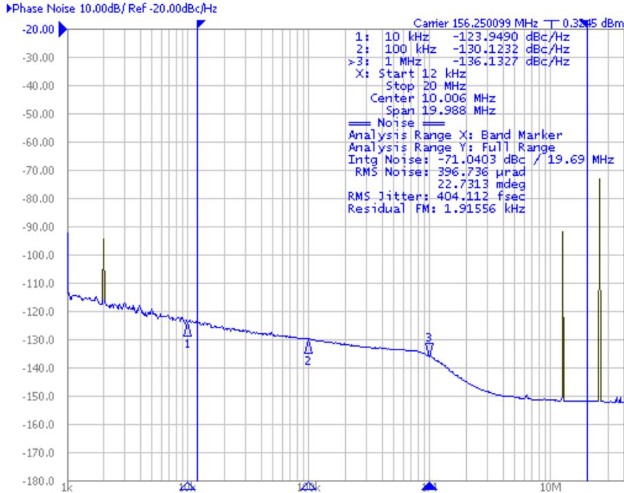
Adding one output at 100MHz causes a 12.5MHz spur but this spur is below -90dBc and does not contribute significantly to the 12K~20M phase jitter. Phase Noise levels at 10KHz, 100KHz and 1MHz are unaffected. This combination is perfect for the 5P49V6913 with two differential outputs.
