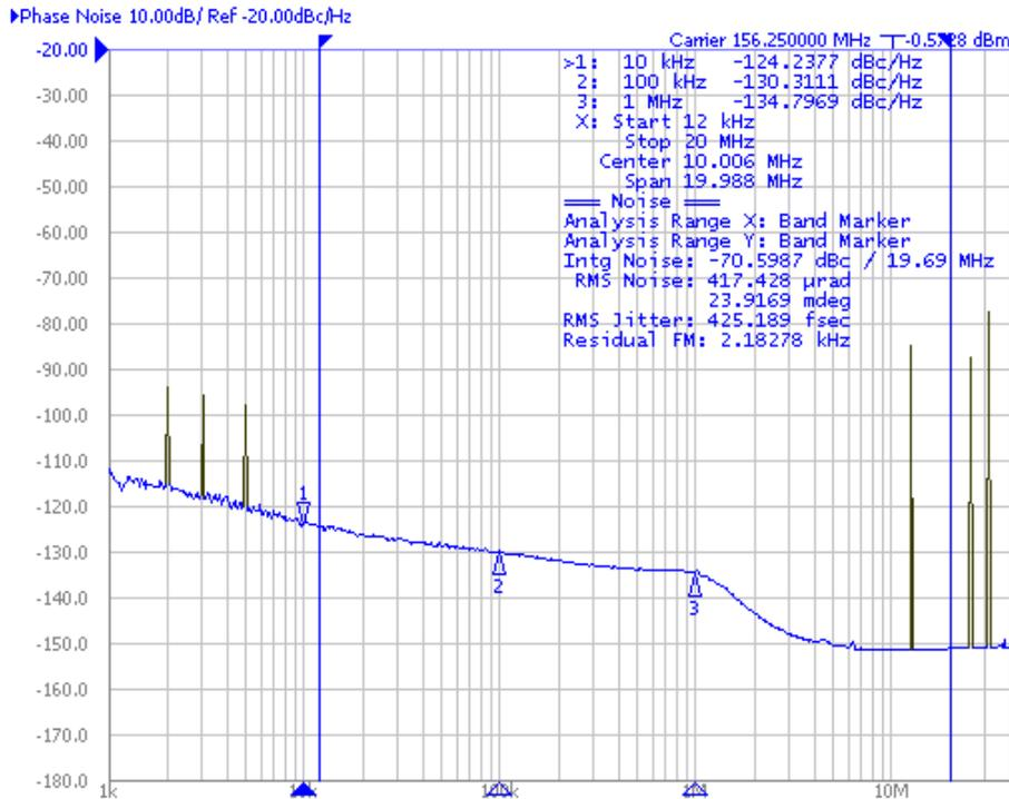
In this case the 12.5MHz spur is a little bit stronger, causing the phase jitter to increase to 425fs. Phase Noise levels at 10KHz, 100KHz and 1MHz are still unaffected. This combination is perfect for the 5P49V6901 with four differential outputs.
