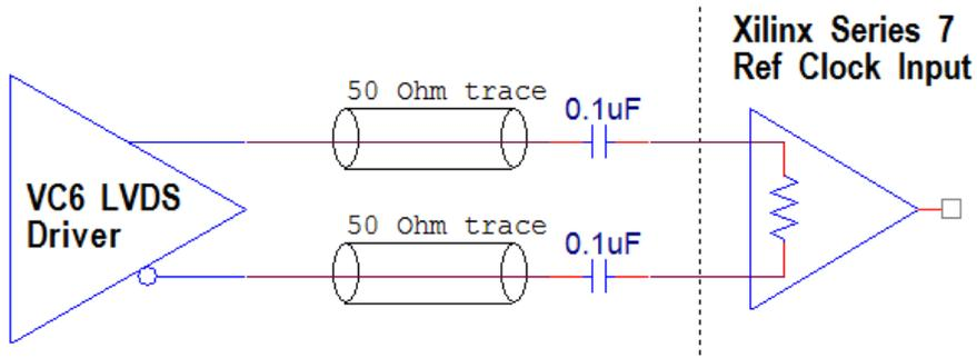
Only the AC coupling capacitors are needed to connect the VersaClock LVDS output to the Xilinx 7 Series FPGA reference clock input.
