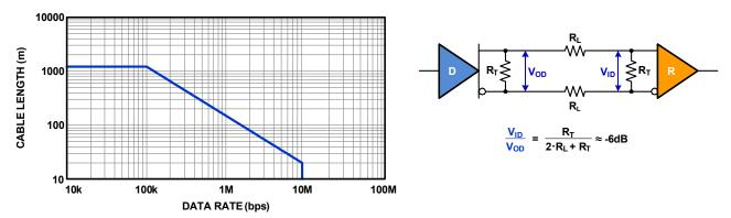
Figure 9. TSB-89 Recommended Maximum Cable Length for Low Data Rates is Based on 6dB Voltage Drop
