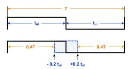
Figure 11. ±20% Pulse Distortion Allows for Easy Data Recovery
