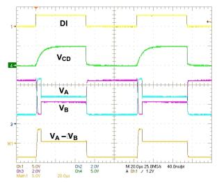
Figure 12. Repeater Waveforms at 20kbps
