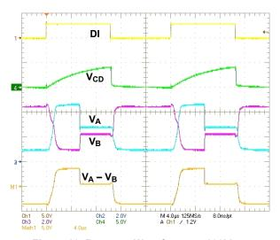
Figure 13. Repeater Waveforms at 100kbps
