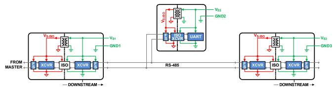
Figure 7. Single Ground Reference Design of a Repeater Link
