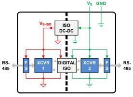
Figure 5. Dual-Isolated HD Repeater
