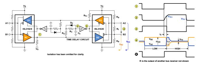
Figure 3. Half-Duplex Repeater with Signal Timing Diagram
