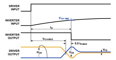
Figure 4. Time Delay Requirement:  $t_D = t_{PLH-MAX} + 0.5 t_{R-MAX}$
