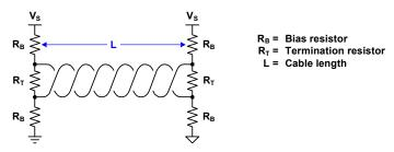
Figure 8. Failsafe Biasing Networks for Long Data Links
