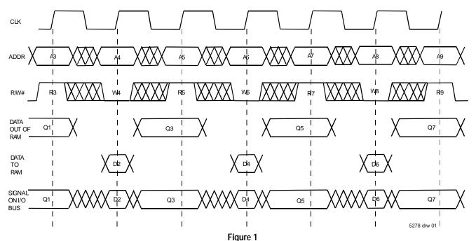
Bus Cycles: Pipelined ZBT, Alternating Reads and Writes
