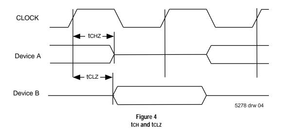
which it is interfacing. An example of this would be an read from an SRAM following a write to the SRAM. In order to avoid bus contention in this case, the ASIC, which is controlling the write, must turn off (tchz) and relinquish control of the bus prior to the SRAM output drivers turning on (tclz) to complete the read.
