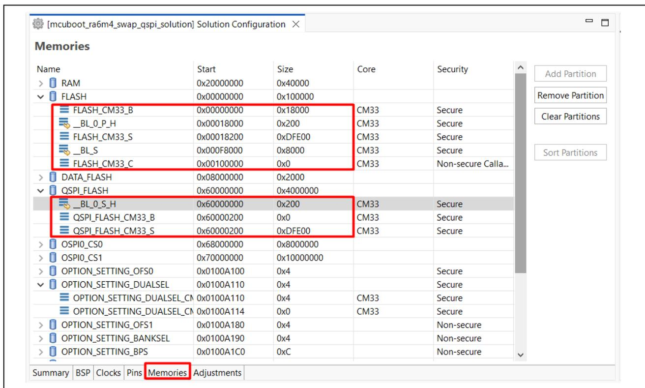
**Figure 48. Memory Partition for Primary and Secondary Image Storage with External Code Flash**
