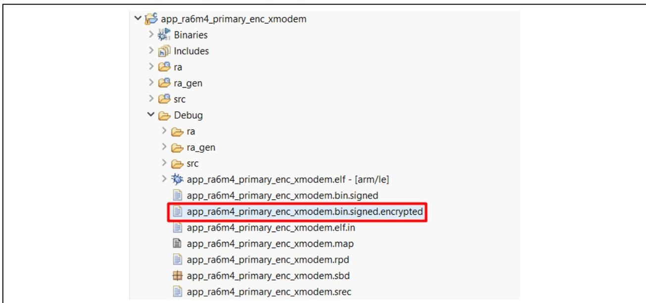
Figure 38. Ensure the Encrypted Binary is Generated
