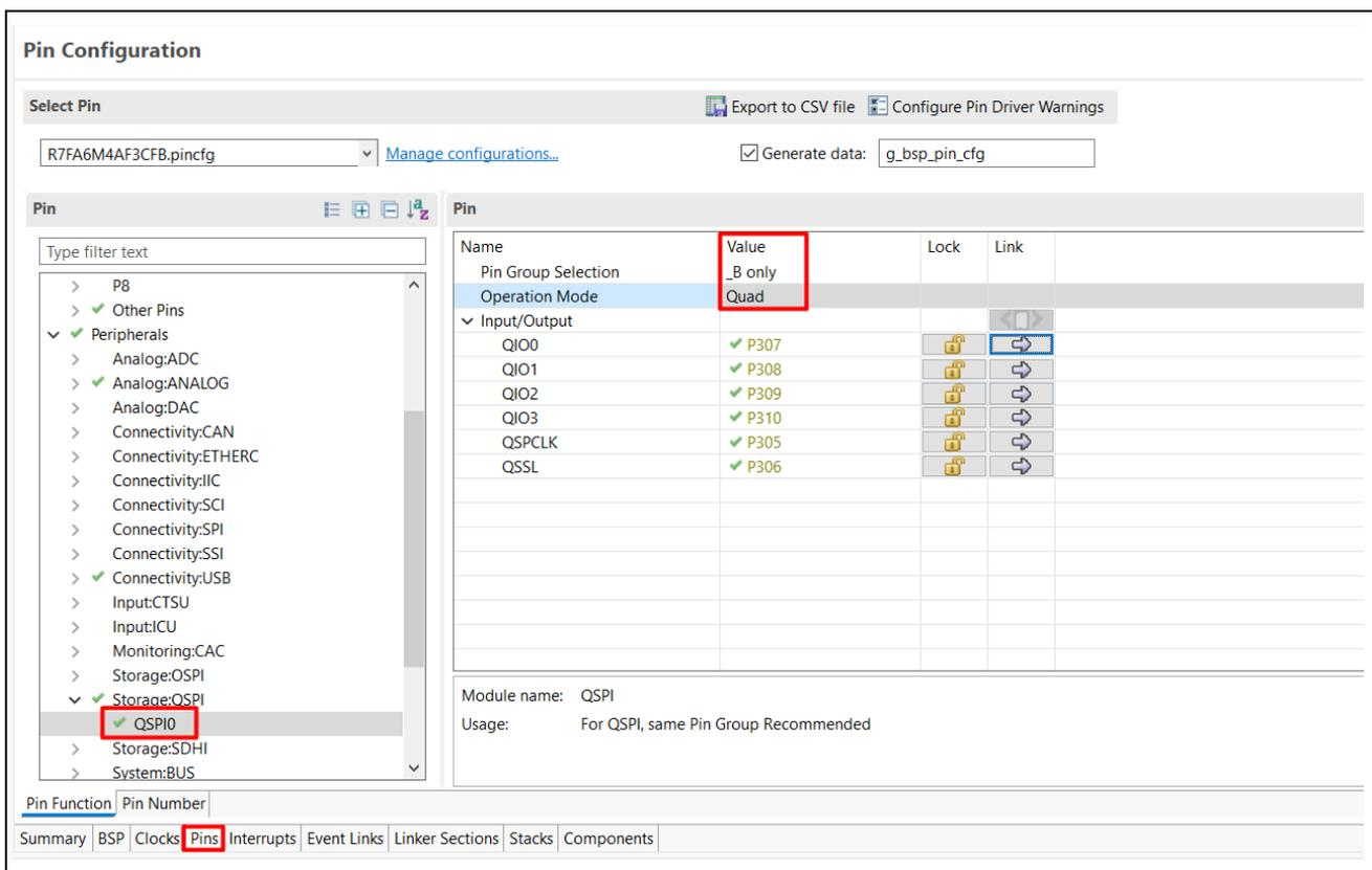
Figure 46. Configure the QSPI Pin and Operation Mode
