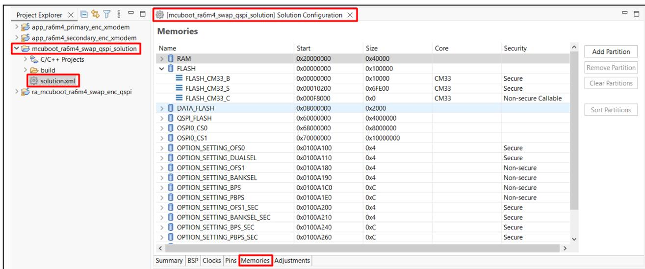
Figure 7. Memory Partition in Solution Project
