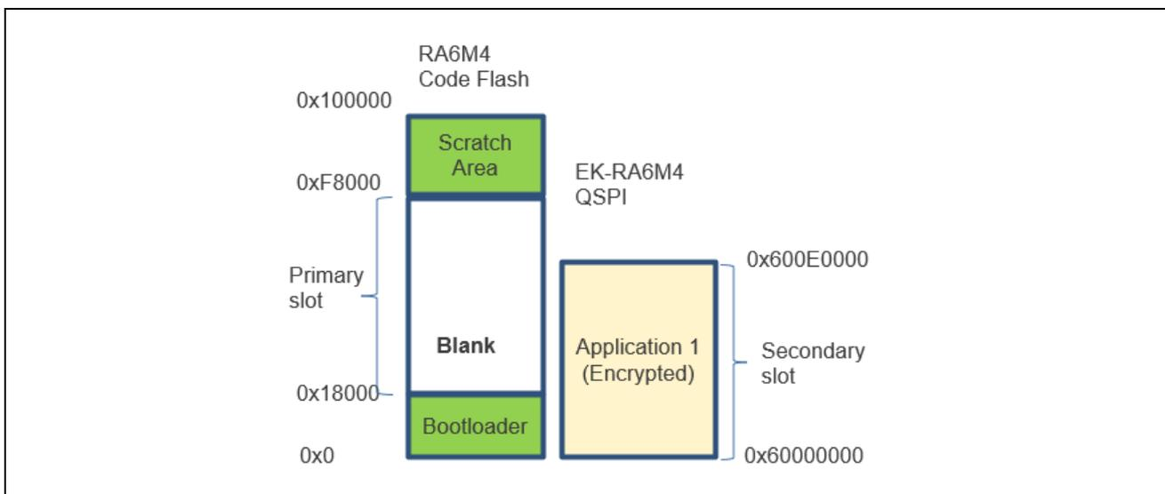
**Figure 43. Using QSPI for Secondary Image Storage**
