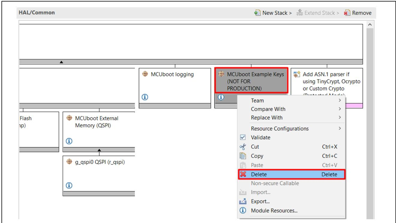
**Figure 61. Delete the MCUboot Example Keys Stack**
