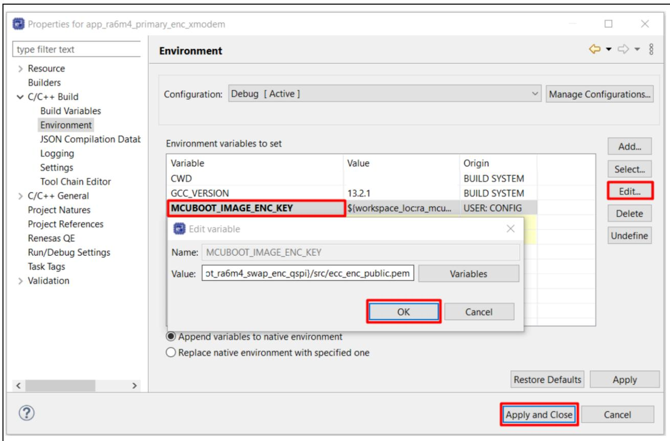
**Figure 67. Configure the Application Project to use the Custom Key for the Image Encryption Process**
