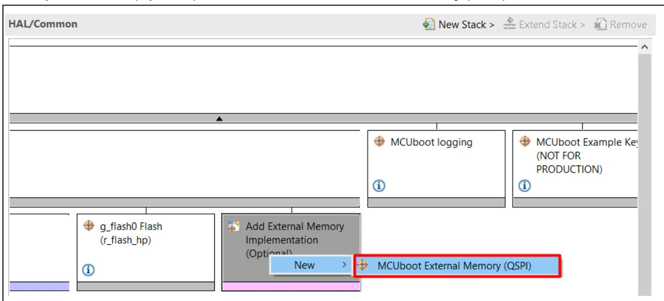
Figure 45. Choose QSPI from the Smart Configurator Stack Tab
