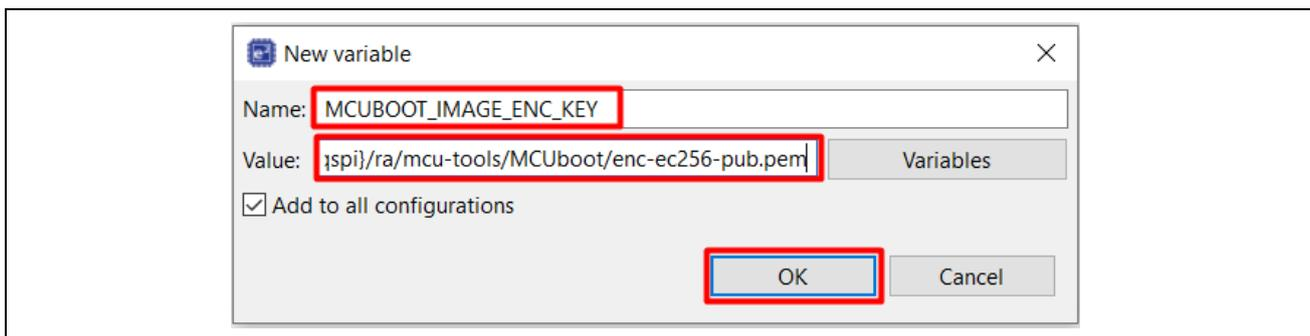
Figure 35. Configure the ECDSA Public Key to be Used in Image Encryption
