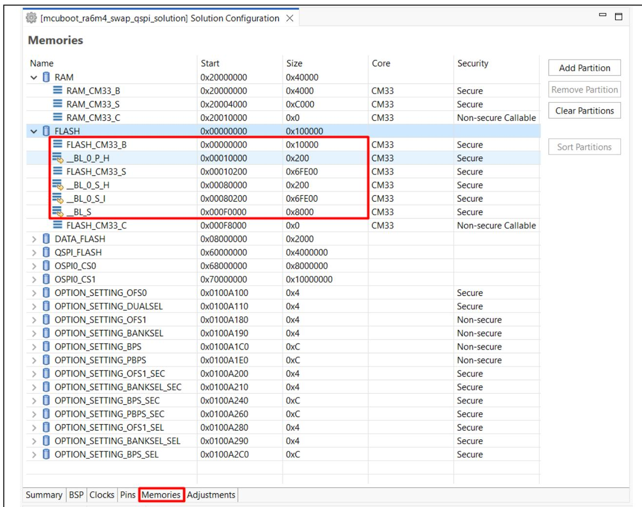
Figure 9. Memory Partition for Primary and Secondary Image Storage with Internal Code Flash
