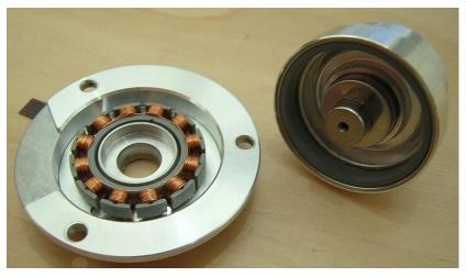
Figure 1: 12 Tooth BLDC Motor
