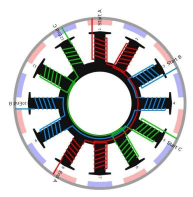
Figure 2: BLDC Motor Coil Placement
