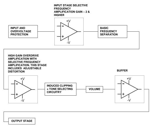
Figure 2: Overview Block Diagram of Overdrive Circuit
