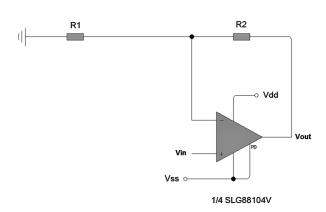
Figure 3: Non-inverting Amplifier Topology
