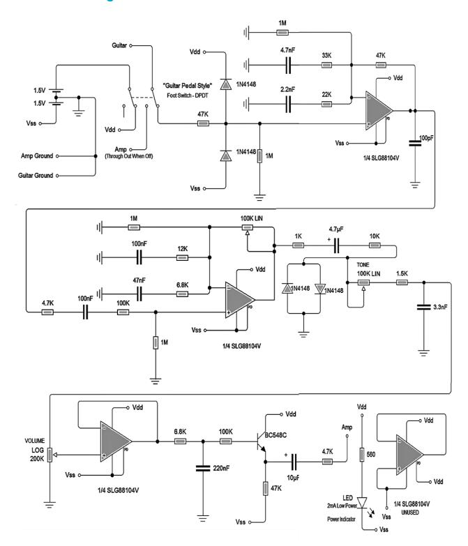
Figure 6: Low Voltage, Low Power Overdrive - Circuit Diagram
