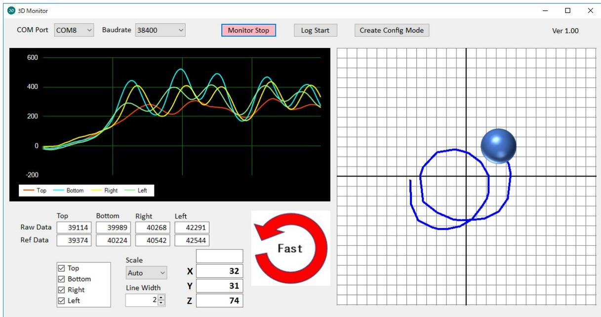
**Figure 4.3 3D Monitor Operation Screen**
