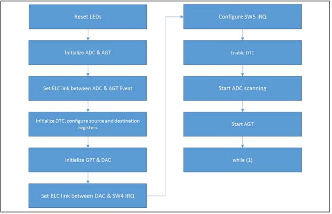
Figure 4 ELC HAL Module Application Project Flow Diagram
