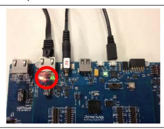
Figure 8. Orange and green Ethernet status LEDs
