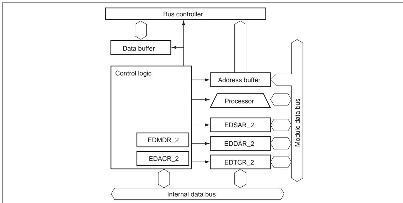
**Figure 2 Block Diagram of EXDMAC**
