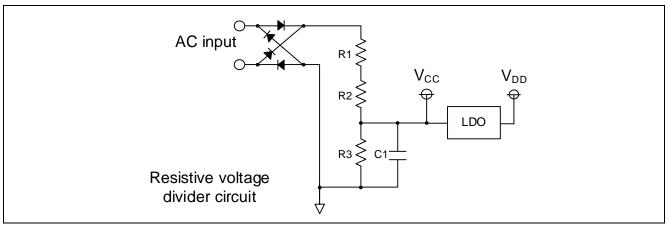
V<sub>CC</sub>: Pre-driver power voltage, V<sub>DD</sub>: MCU power voltage (5 V)
