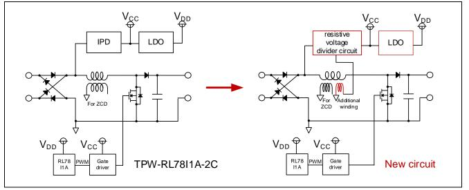
Note: The ZCD auxiliary winding and additional auxiliary winding can be used as one winding depending on conditions.
