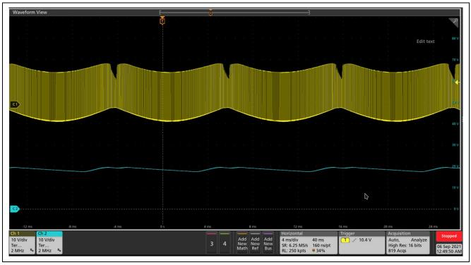
Figure 3 - 9 Auxiliary Winding Output Voltage (at 260 VAC, Upper Waveform: Auxiliary Winding Voltage, Lower Waveform: Vcc)
