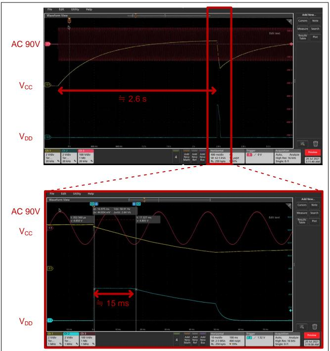
Figure 3 - 5 V<sub>CC</sub>/V<sub>DD</sub> Voltage Waveforms (R1, R2 = 68 k $\Omega$ , R3 = 15 k $\Omega$ , C1 = 47  $\mu$ F, 5 mA Load Connected to V<sub>DD</sub>)
