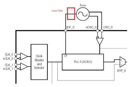
Figure 7. 8V19N491-24 VCXO Phase Lock Loop Block Diagram
