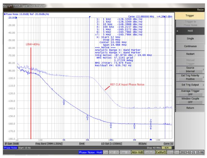
Figure 20. PLL Output Phase Noise with Optimized Loop Bandwidth
