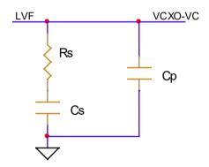
Figure 8. Typical 2nd Order Loop Filter
