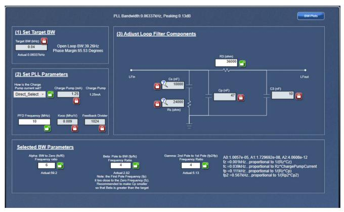
Figure 10. Loop Filter Calculation Tool Example
