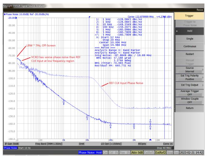
Figure 18. PLL Output Phase Noise for Loop Bandwidth Set Too Low
