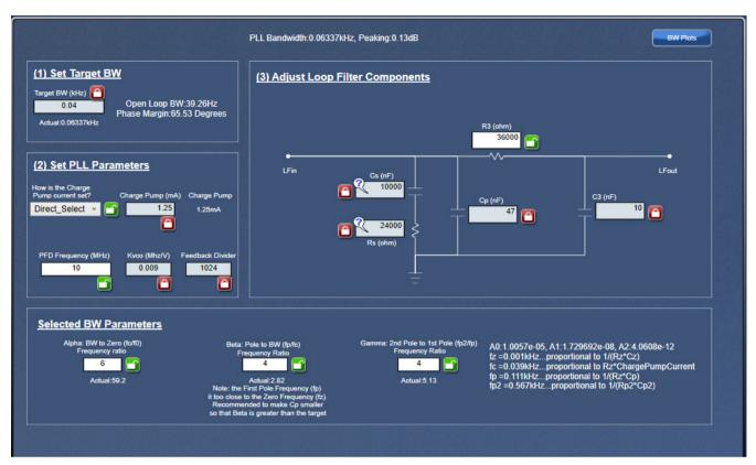
Figure 19. Loop Bandwidth = 40Hz and Phase Margin = 65 degrees
