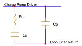
Figure 5. Typical 2nd Order Loop Filter
