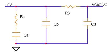
Figure 9. Typical 3rd Order Loop Filter
