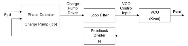
Figure 1. Basic PLL Block Diagram
