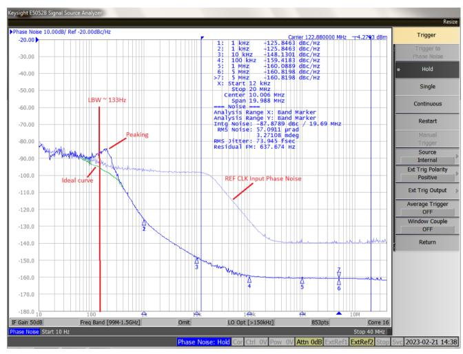
Figure 16. PLL Output Phase Noise for Loop Bandwidth Set Too High
