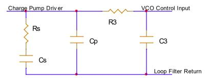
Figure 6. Typical 3rd Order Loop Filter
