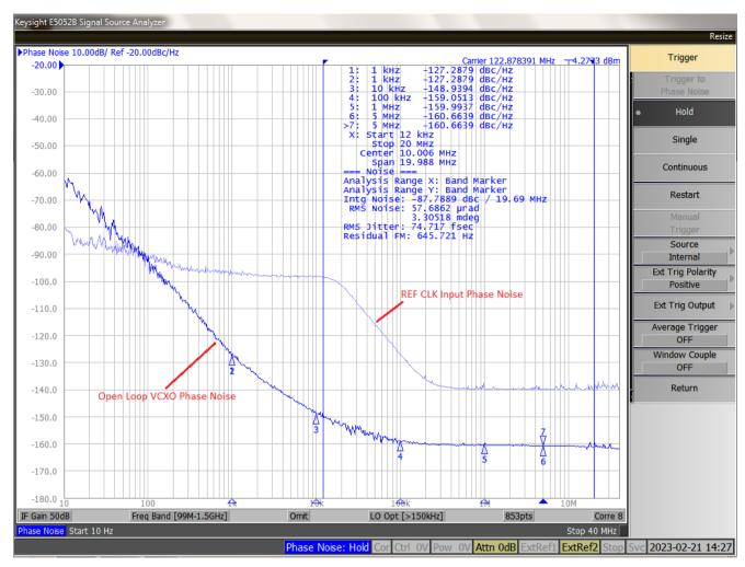
Figure 14. Open Loop VCXO Phase Noise vs AFG3252 REF CLK Input – both at 122.88MHz
