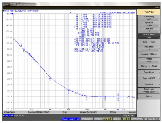
Figure 13. VG3225EFN VCXO Open Loop Phase Noise Performance
