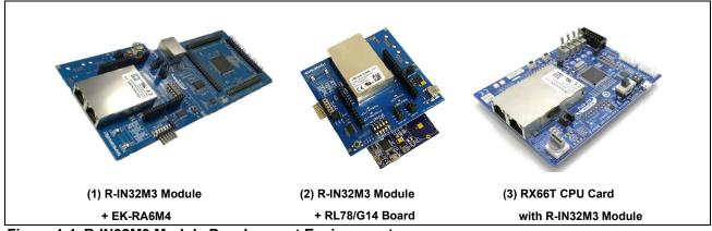
Figure 1-1 R-IN32M3 Module Development Environment
