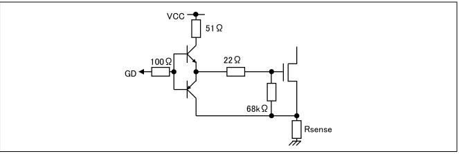
Figure 3 Drive circuit example
