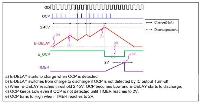
Figure 9 Over-current Error Operation
