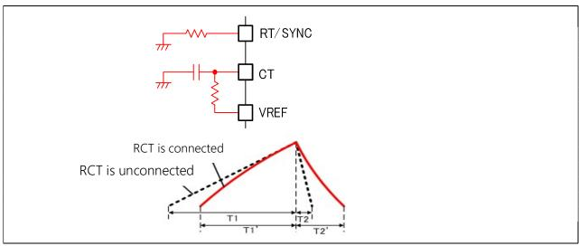
Figure 16 Max. Duty limit circuit
