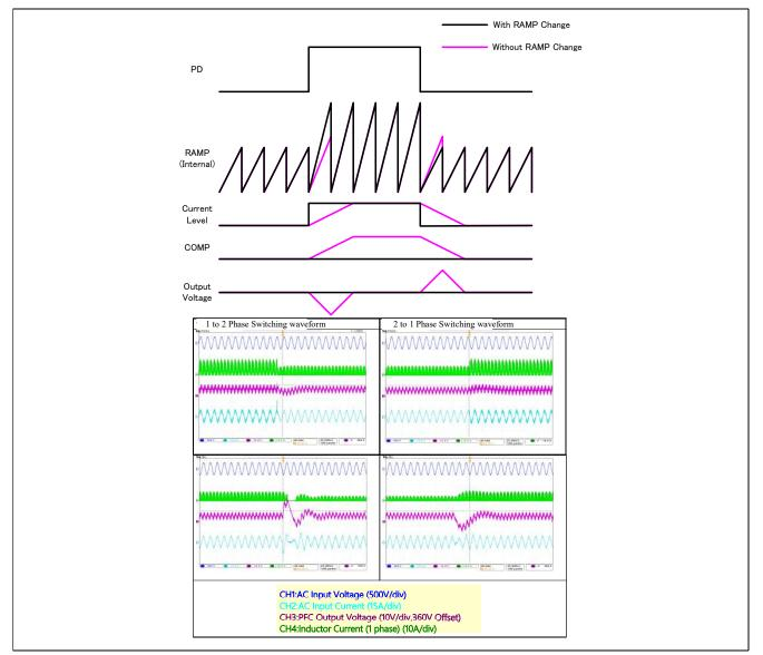
Figure 6 Operation at Phase Drop Switching
