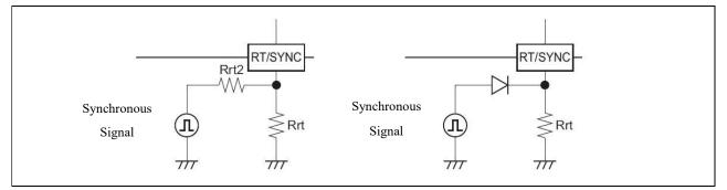
Figure 12 Synchronous Signal Input
