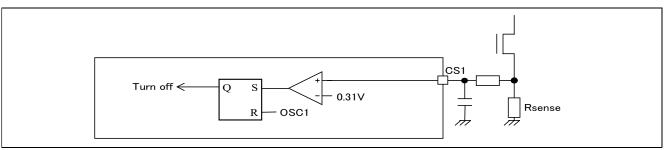
Figure 2 Over-current protection
