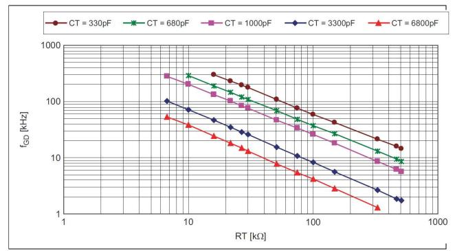
Figure 13 Operating Frequency Characteristics
