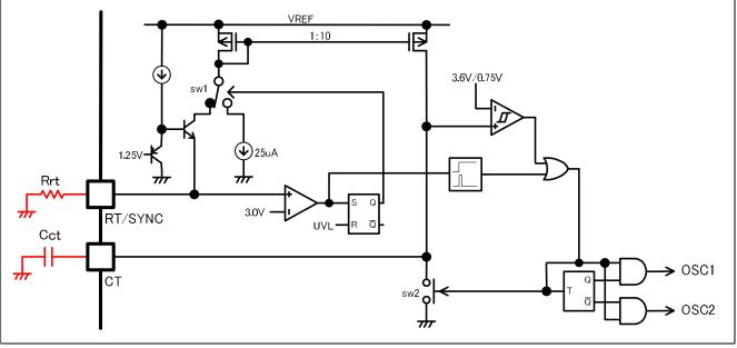
Figure 10 Outline of Synchronous Circuits
