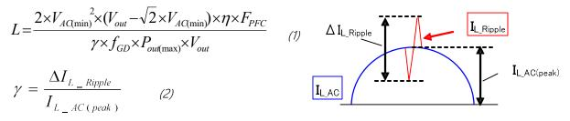
Vac(min) : Effective value of minimum input voltage [V(rms)]
