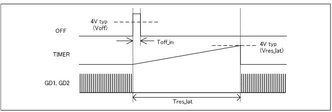
Figure 3.6 OFF Function Operation
