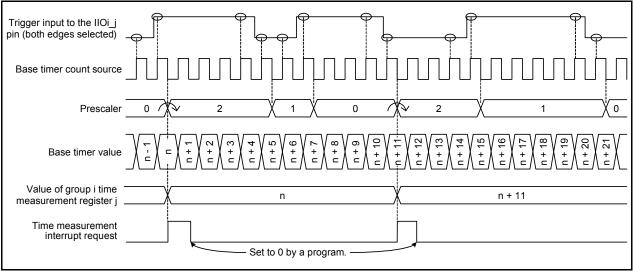
Figure 3.6 Prescaler Timing Diagram
