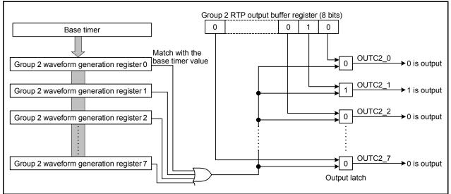
Figure 3.14 Outline of Parallel RTP Output Mode
