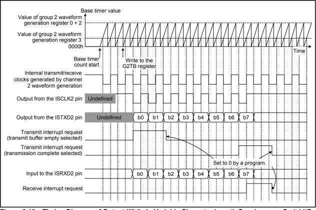
Figure 3.16 Timing Diagram of Output While In Variable Character Length Synchronous Serial I/O Mode
