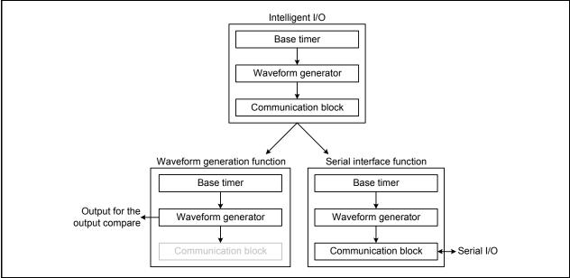
Figure 1.2 Overview of the Intelligent I/O for Groups Embedded With Waveform Generation and Serial Interface Function
