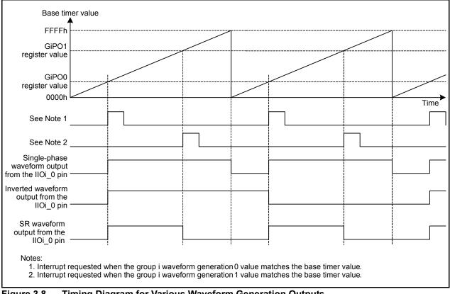
Figure 3.8 Timing Diagram for Various Waveform Generation Outputs
