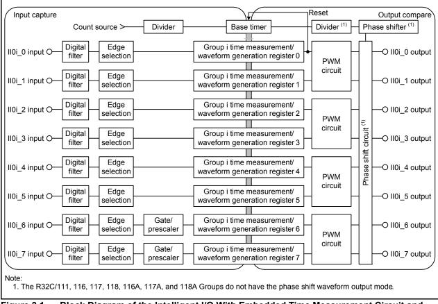
Figure 3.1 Block Diagram of the Intelligent I/O With Embedded Time Measurement Circuit and Waveform Generation Function
