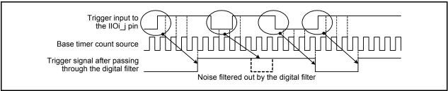
Figure 3.4 Digital Filter Timing Diagram
