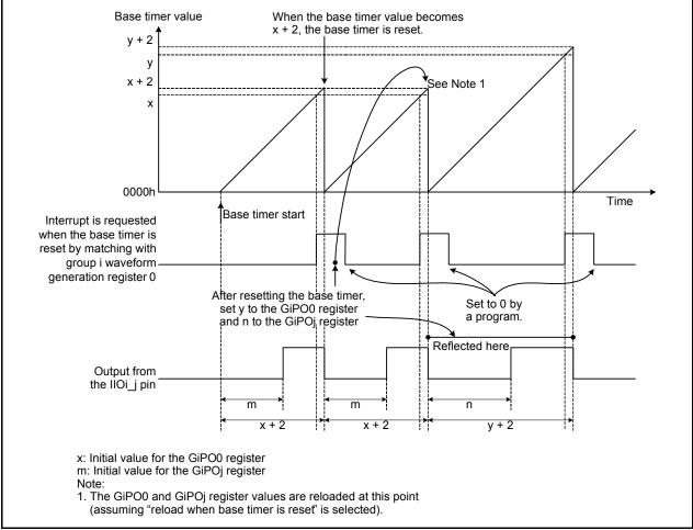
Figure 3.10 Timing Diagram of 16-Bit PWM Output
