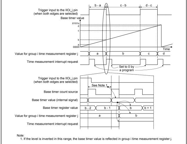
Figure 3.3 Timing Diagram of the Time Measurement Function
