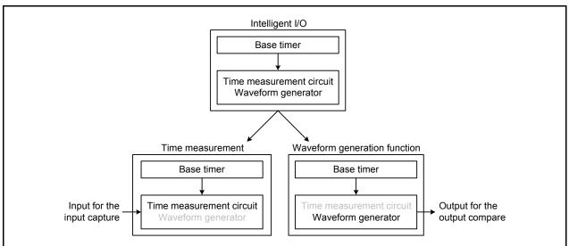
Figure 1.1 Overview of the Intelligent I/O for Groups Embedded With Time Measurement and Waveform Generation
