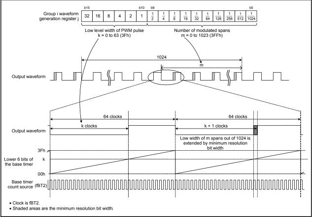
Figure 3.11 Timing Diagram of Bit Modulation PWM Output Mode
