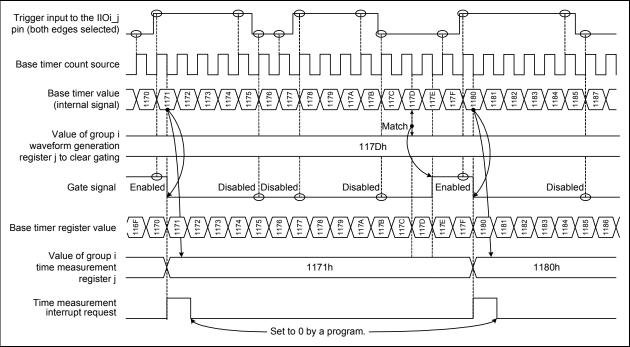
Figure 3.5 Timing Diagram of Gating
