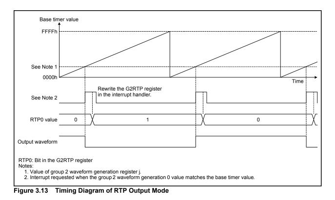
Note that the RTP output mode can only be used with the R32C/111, 116, 117, 118, 116A, 117A, and 118A Groups.
