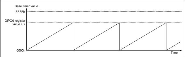
Figure 3.9 Base Timer Reset Timing Diagram
