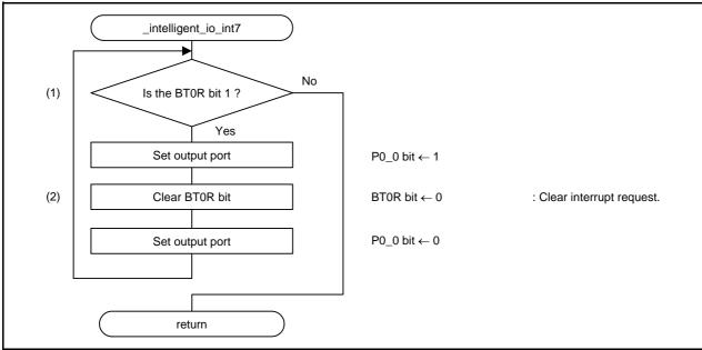
Figure 5.5 Intelligent I/O Interrupt Handling
