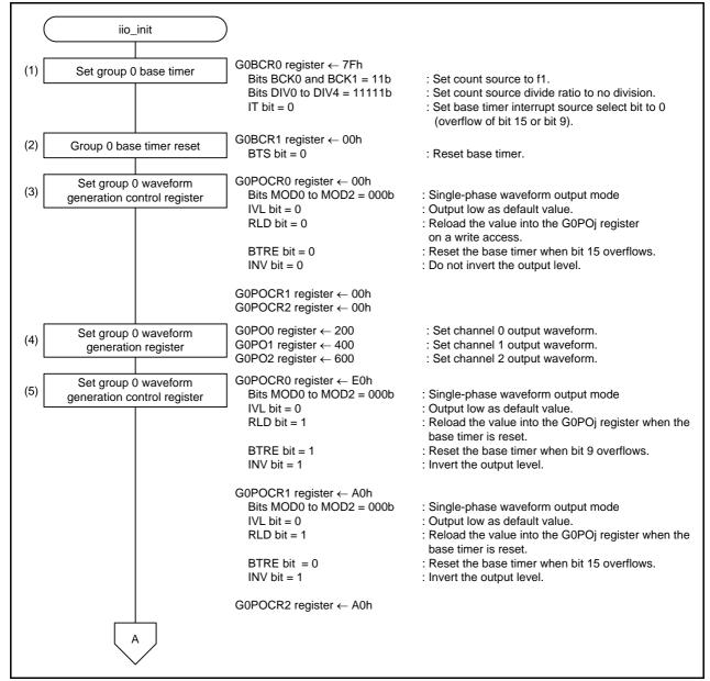
Figure 5.3 Intelligent I/O Initialization (1/2) (j = 0 to 2)
