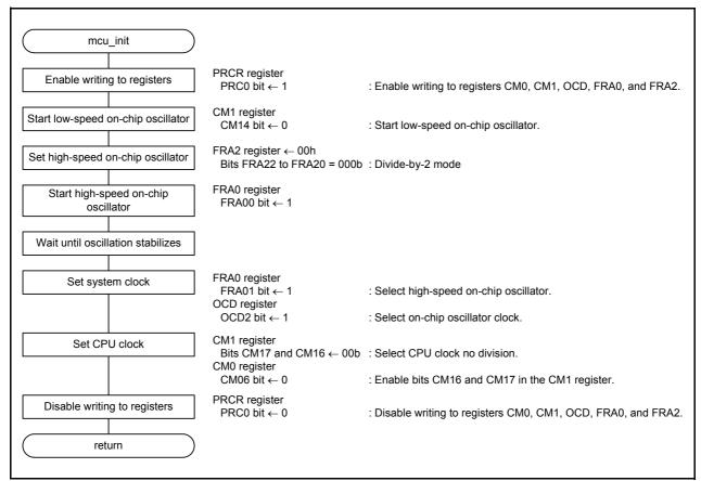
Figure 4.3 System Clock Setting
