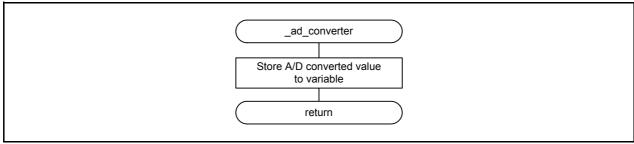
Figure 4.5 A/D Conversion Interrupt Handling
