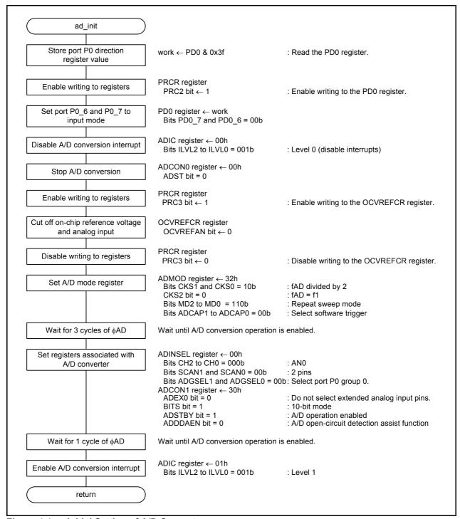
Figure 4.4 Initial Setting of A/D Converter
