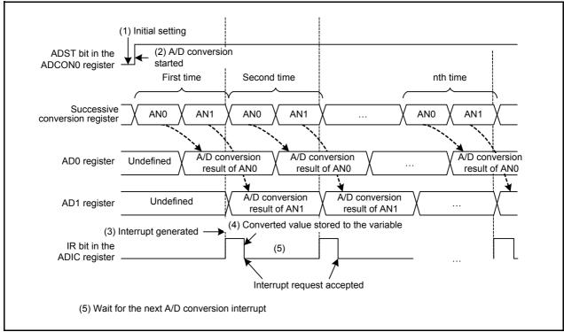
Figure 4.1 Timing Diagram in Repeat Sweep Mode
