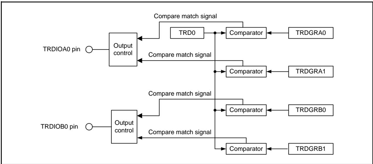
Figure 3.1 Block Diagram
