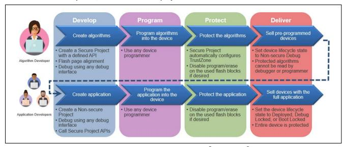
Figure 4. IP Protection using Arm® TrustZone®
