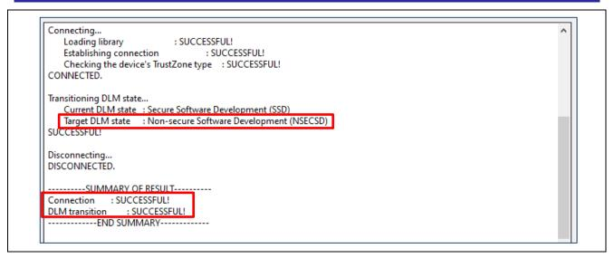
Figure 59. Result: Transition from SSD to NSECSD
