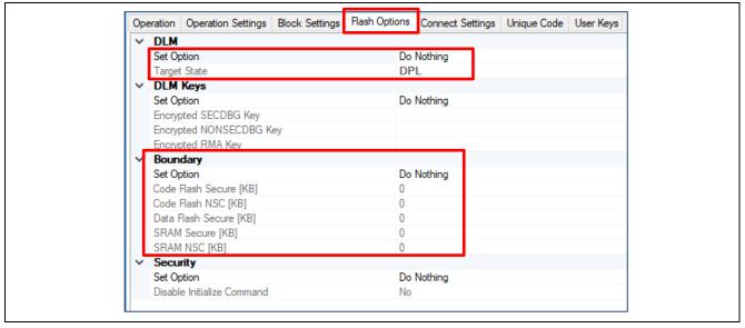
Figure 96. Operation Settings for Non-secure Project Binary Download
