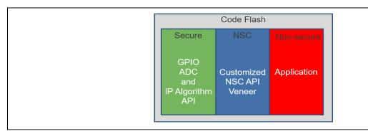
Figure 47. Sensor Algorithm IP Protection
