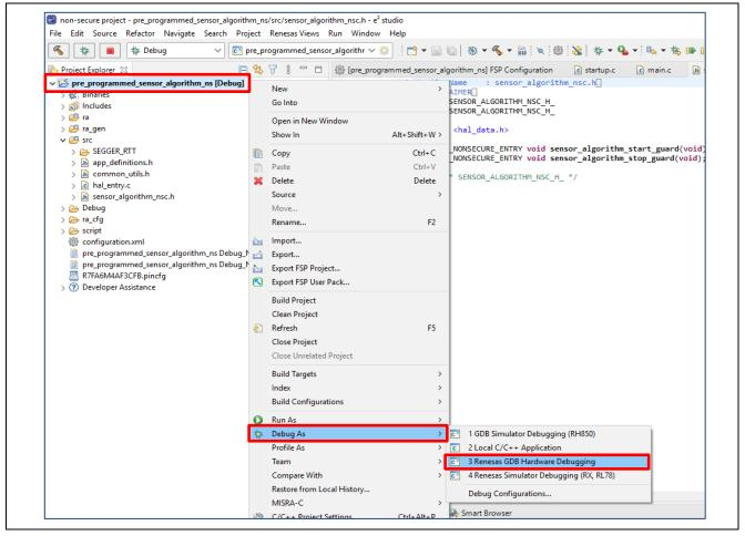
Figure 62. Download and Run the Non-secure Project
