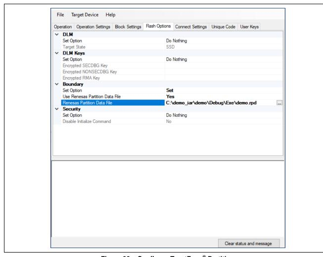
Figure 98. Configure TrustZone® Partition
