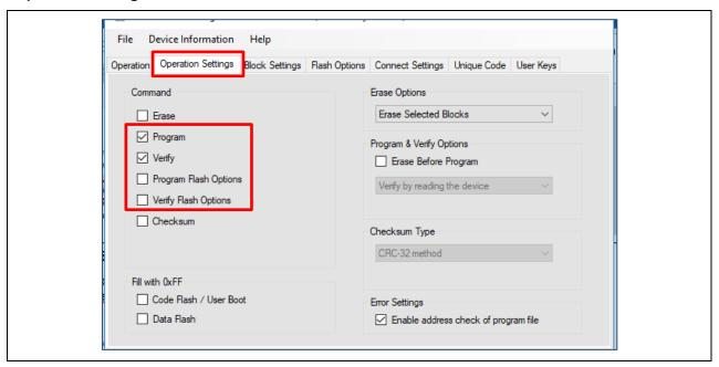
Figure 95. Operation Settings for Non-secure Project Binary Download
