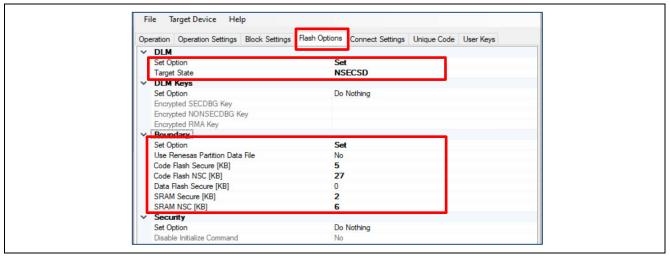
Figure 92. Setup for the IDAU Region
