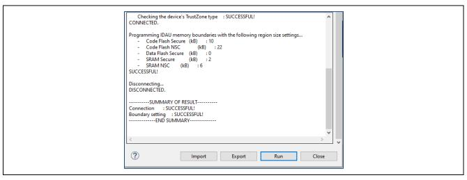
Figure 84. IDAU Region is Configured Correctly
