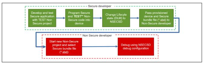
Figure 42. Development Flow for Developing in NSECSD State
