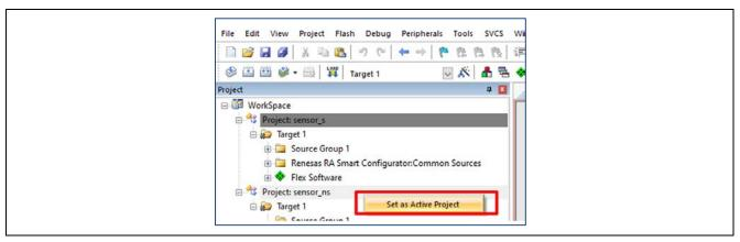
Figure 85. Set the Non-secure Project as the Active Project
