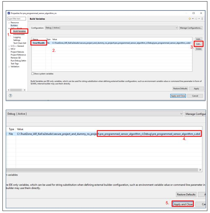
Figure 61. Referencing the Secure Bundle
