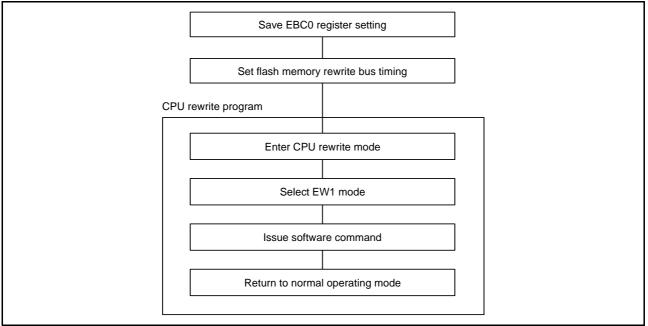
Figure 3.3 CPU Rewrite Mode (EW1 Mode) Execution Flow
