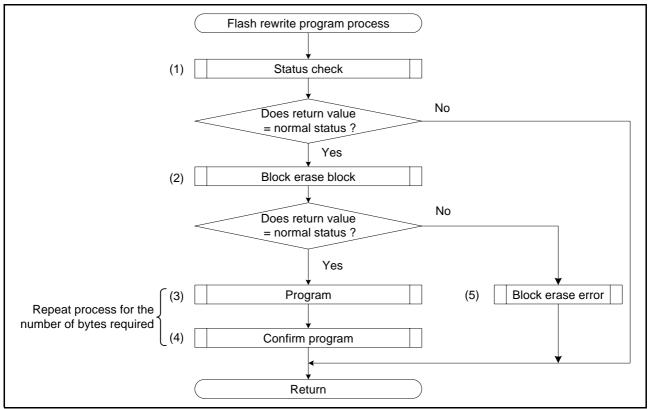
Figure 4.3 shows the process flowchart of the CPU rewrite program. Repeat program process for data to be written.
