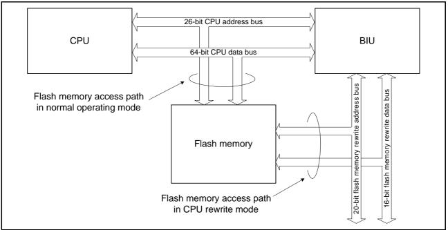
Figure 3.1 Flash Memory Access Path in CPU Rewrite Mode
