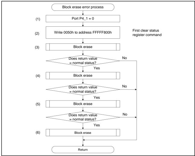
Figure 4.5 Block Erase Error Function
