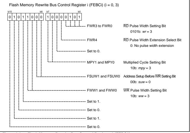
Figure 3.2 Flash Memory Rewrite Bus Control Register 0 (FEBC0)
