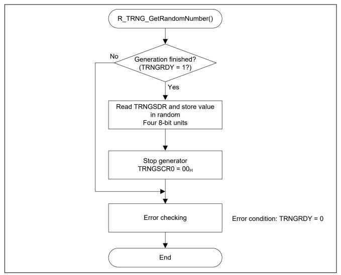
Figure 2.2 R\_TRNG\_GetRandomNumber Function Processing Flowchart
