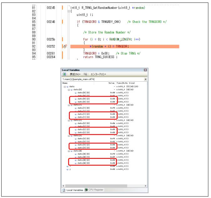
Figure 4.3 Break Occurs R\_TRNG\_GetRandomNumber while Is Running
