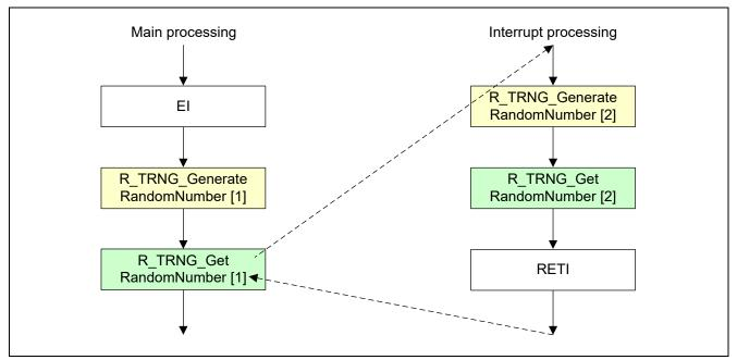
Figure 4.2 Interrupt Occurs while R\_TRNG\_GetRandomNumber Is Running
