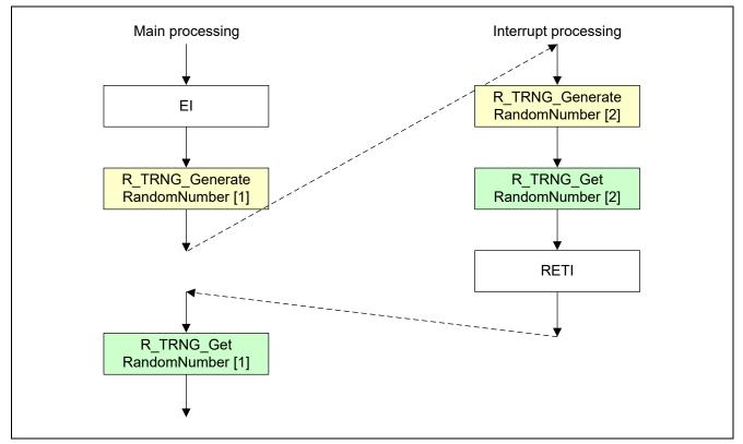
Figure 4.1 Interrupt Occurs after R\_TRNG\_GenerateRandomNumber Runs
