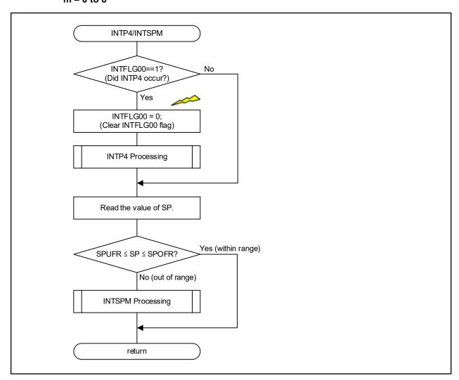
Figure 2-1 INTP4/INTSPM Interrupt Judgement Example (INTP4 occurs continuously)
