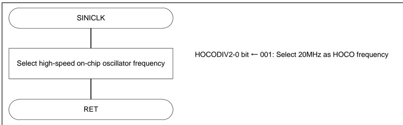
**Figure 5.6 Clock Generation Circuit Settings**
