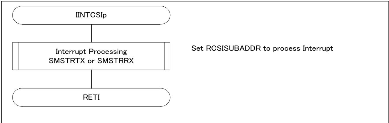
Figure 5.16 INTCSI00 Interrupt Processing
