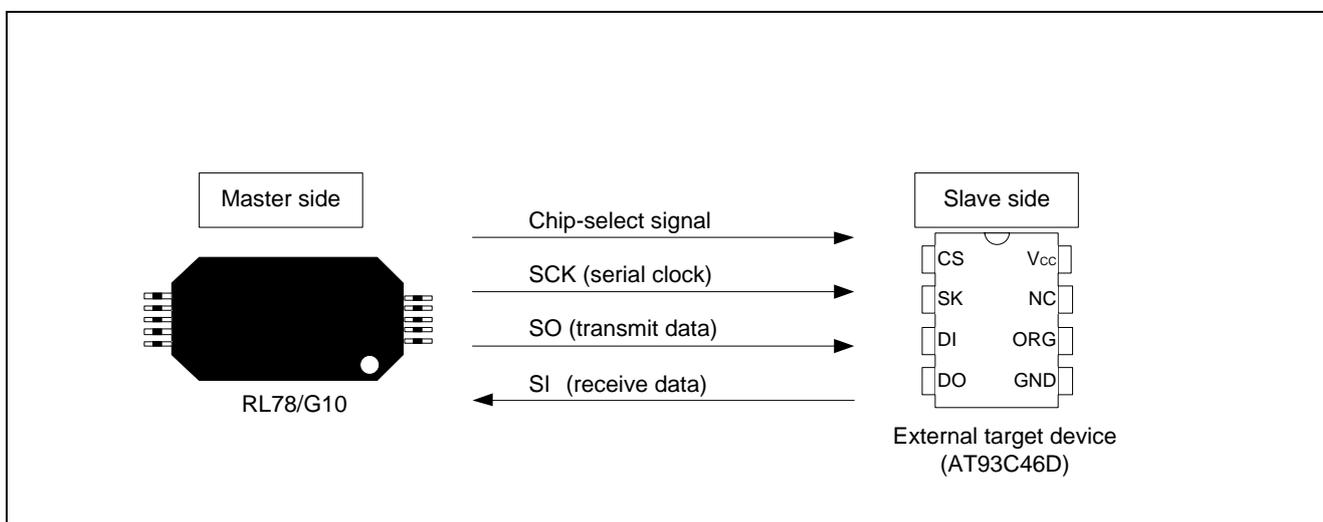
**Figure 1.1 Microwire Operating Configuration**
