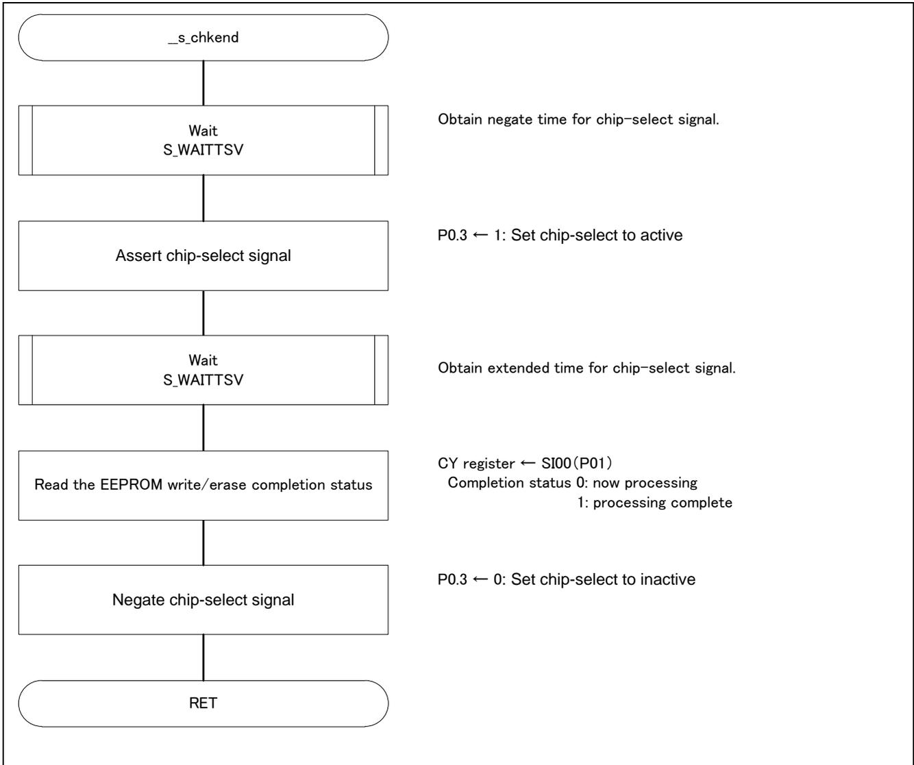
Figure 5.15 EEPROM Data Write/Erase All Completion Status Read Processing
