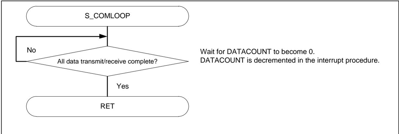
**Figure 5.21 All Data Transmit/Receive Complete Wait Processing**
