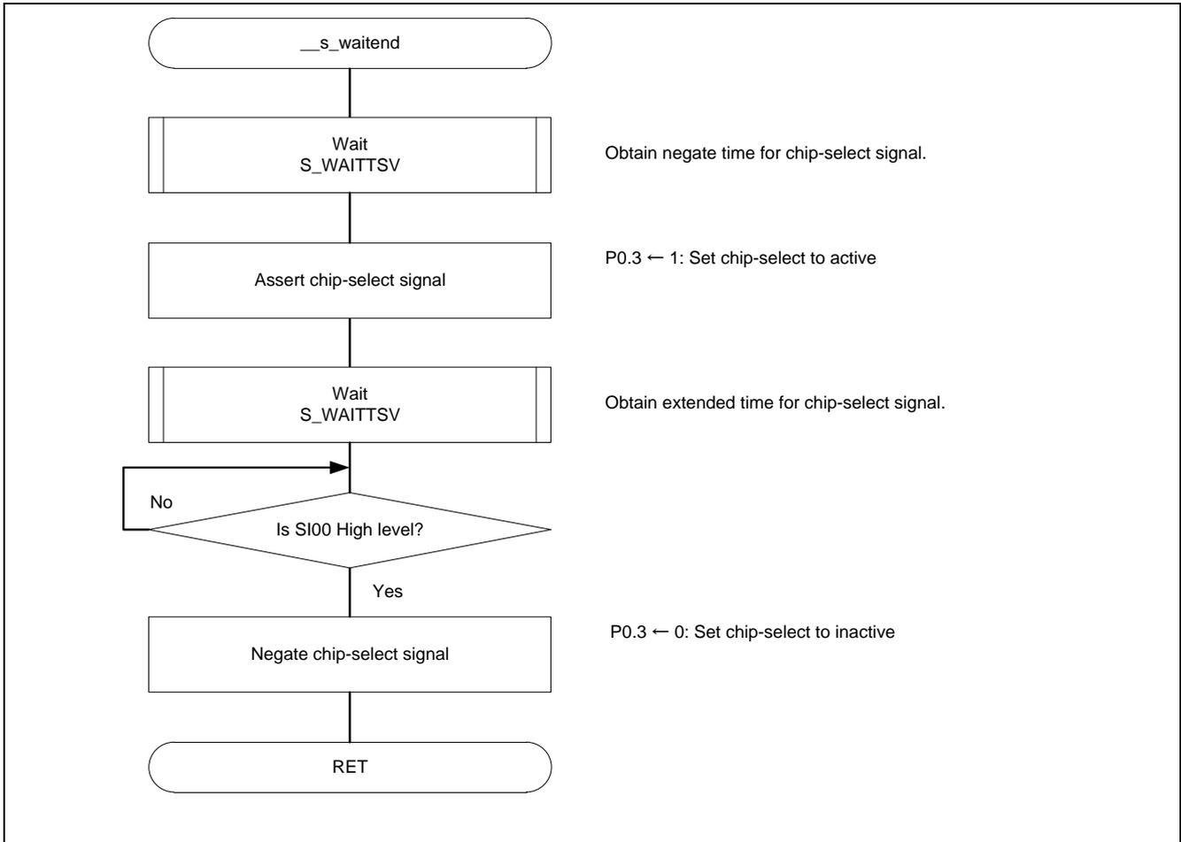
Figure 5.14 EEPROM Data Write/Erase All Areas Completion Wait Processing
