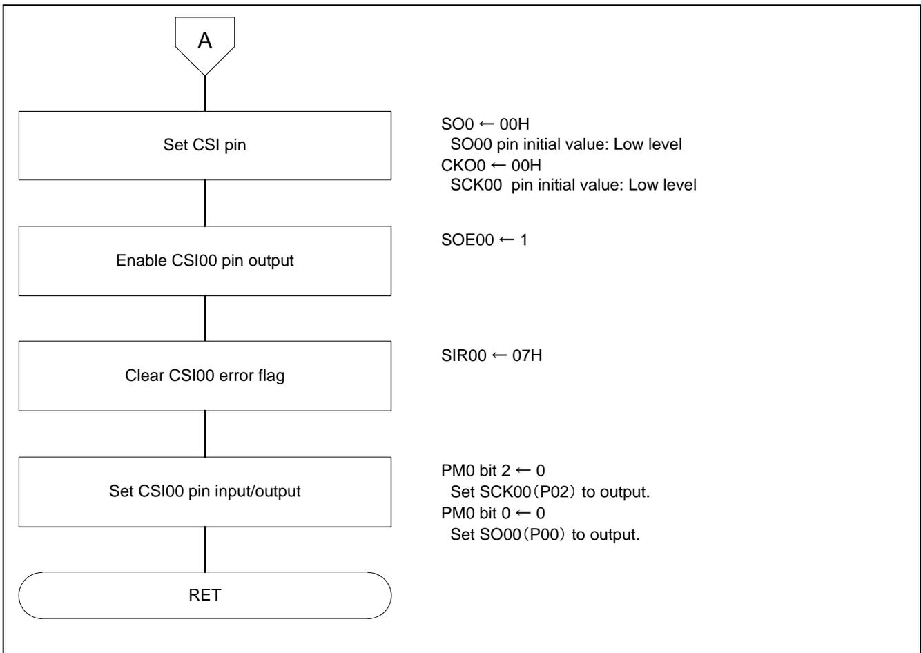
Figure 5.7 Serial Array Unit Setting (2/2)
