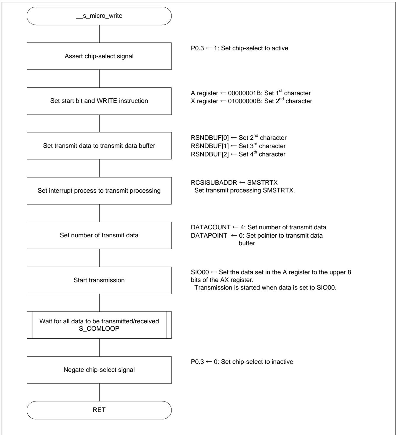
Figure 5.10 Data Write Process to Specified EEPROM Address
