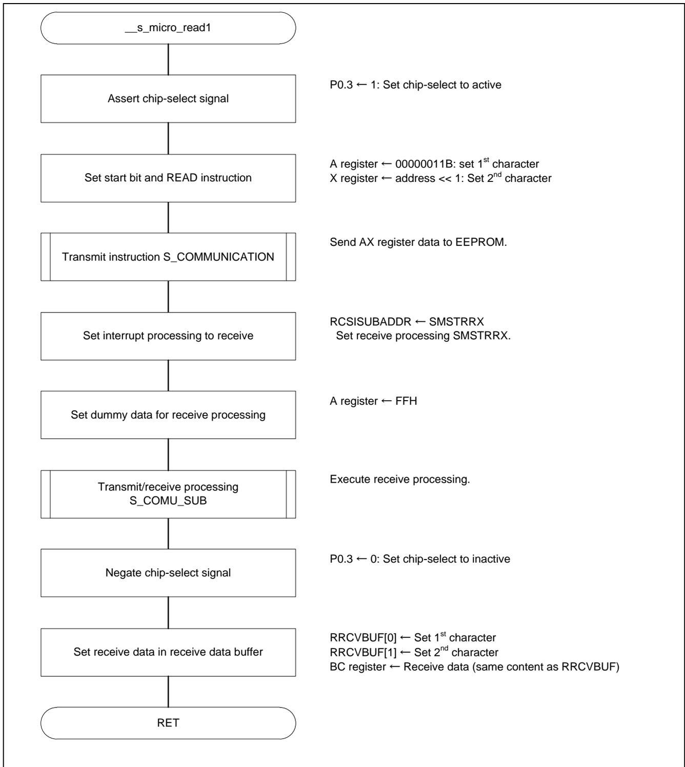
Figure 5.9 Data Read Process from Specified EEPROM Address
