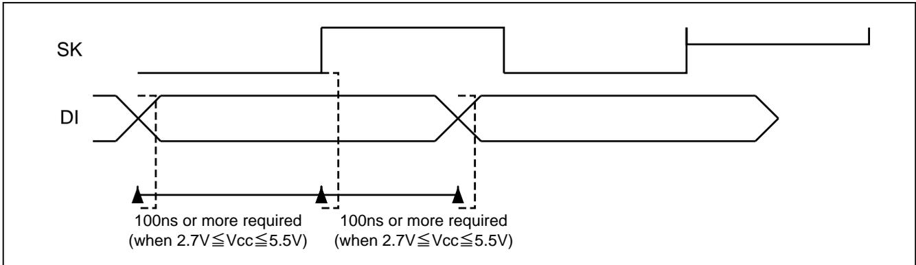
**Figure 1.3 DI Pin Timing Chart**
