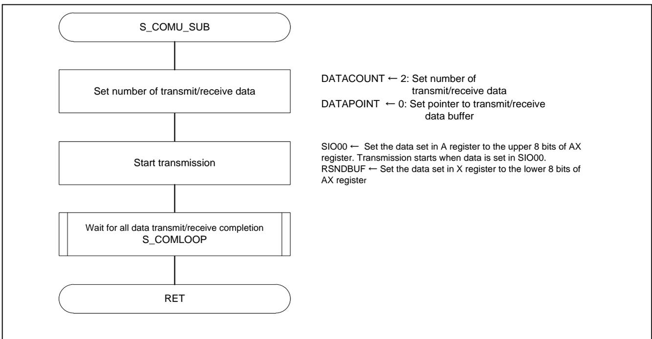
Figure 5.20 EEPROM Transmit/Receive Processing
