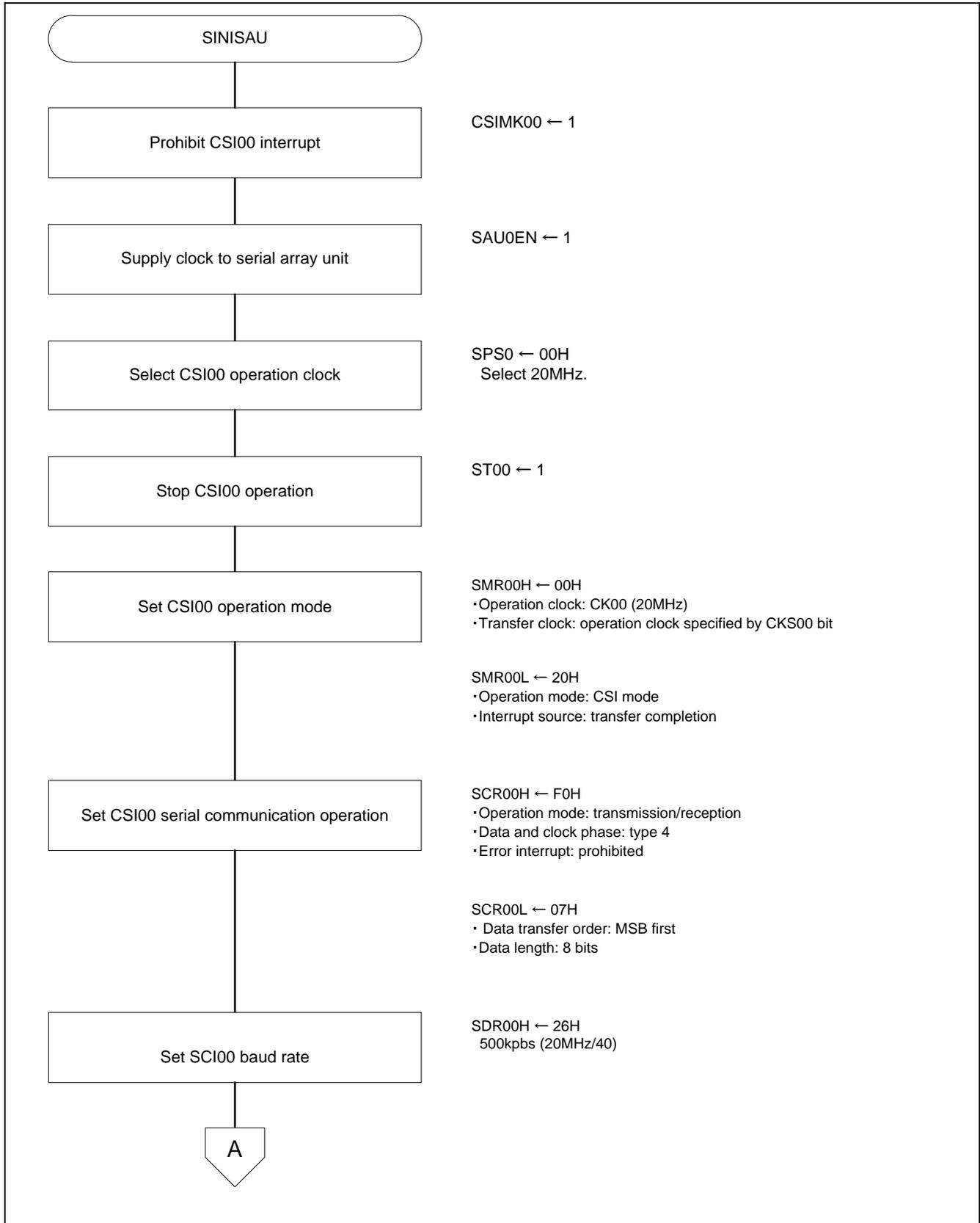
Figure 5.7 Serial Array Unit Setting (1/2)
