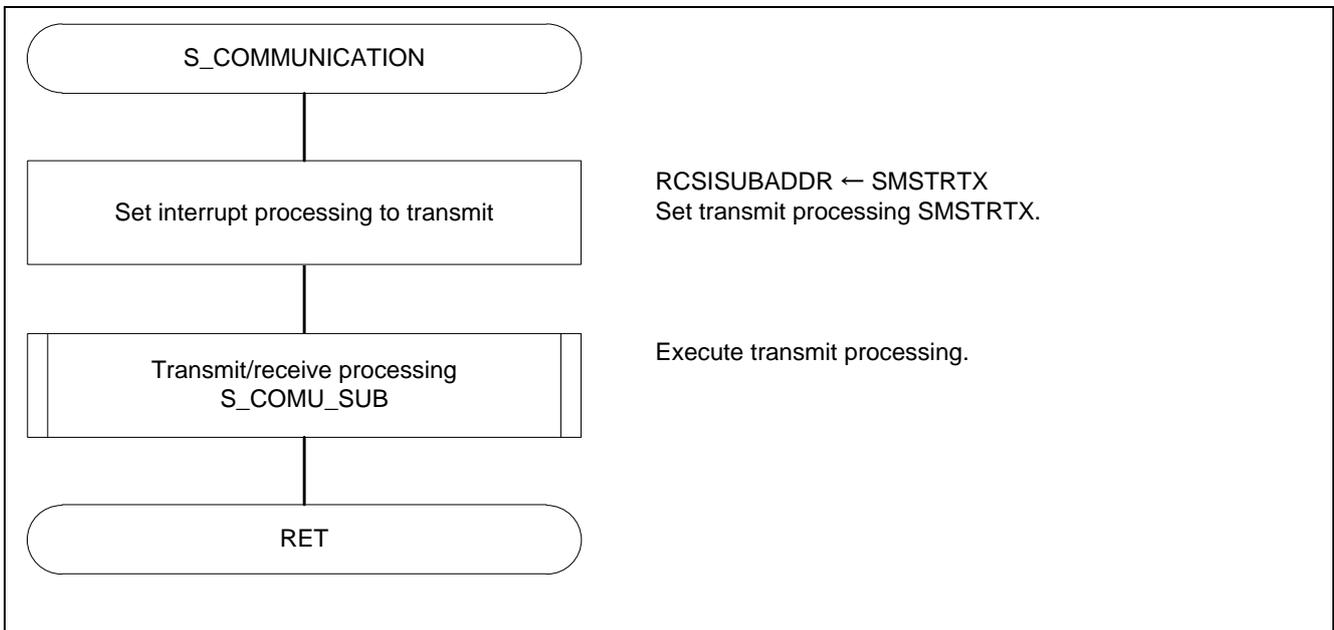
Figure 5.19 EEPROM Instruction Transmit Processing
