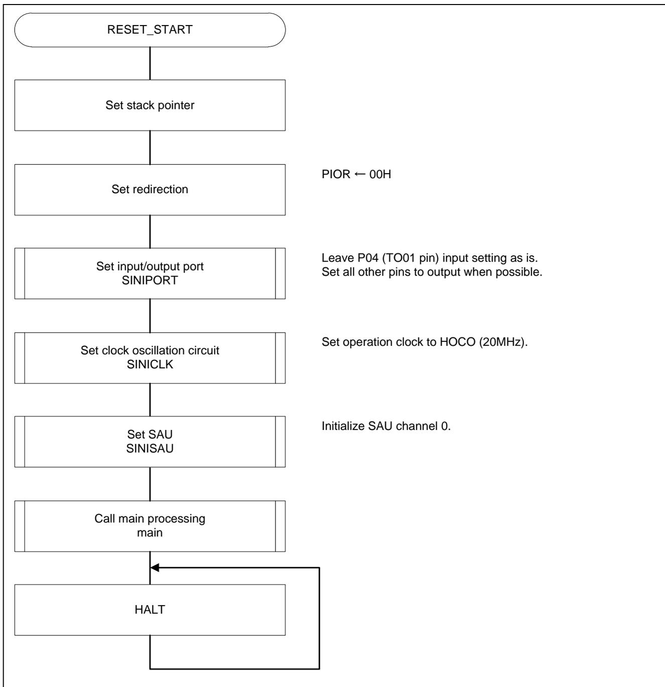
Figure 5.4 CPU Initialization Function
