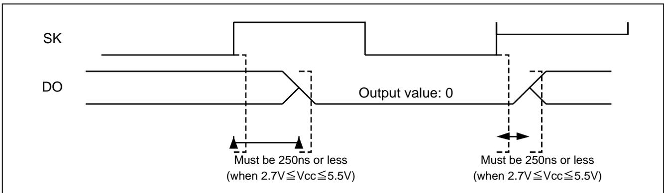
**Figure 1.4 DO Pin Timing Chart**
