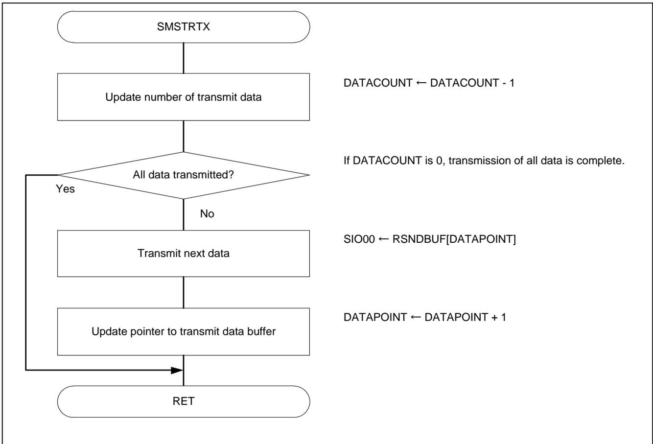
Figure 5.17 Transmit Processing
