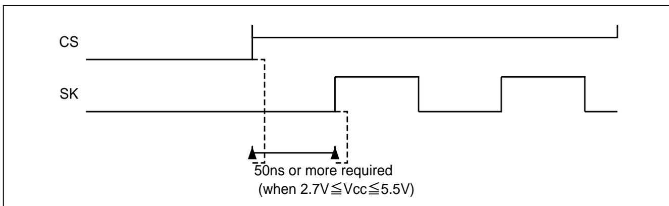
**Figure 1.2 CS Pin Timing Chart**
