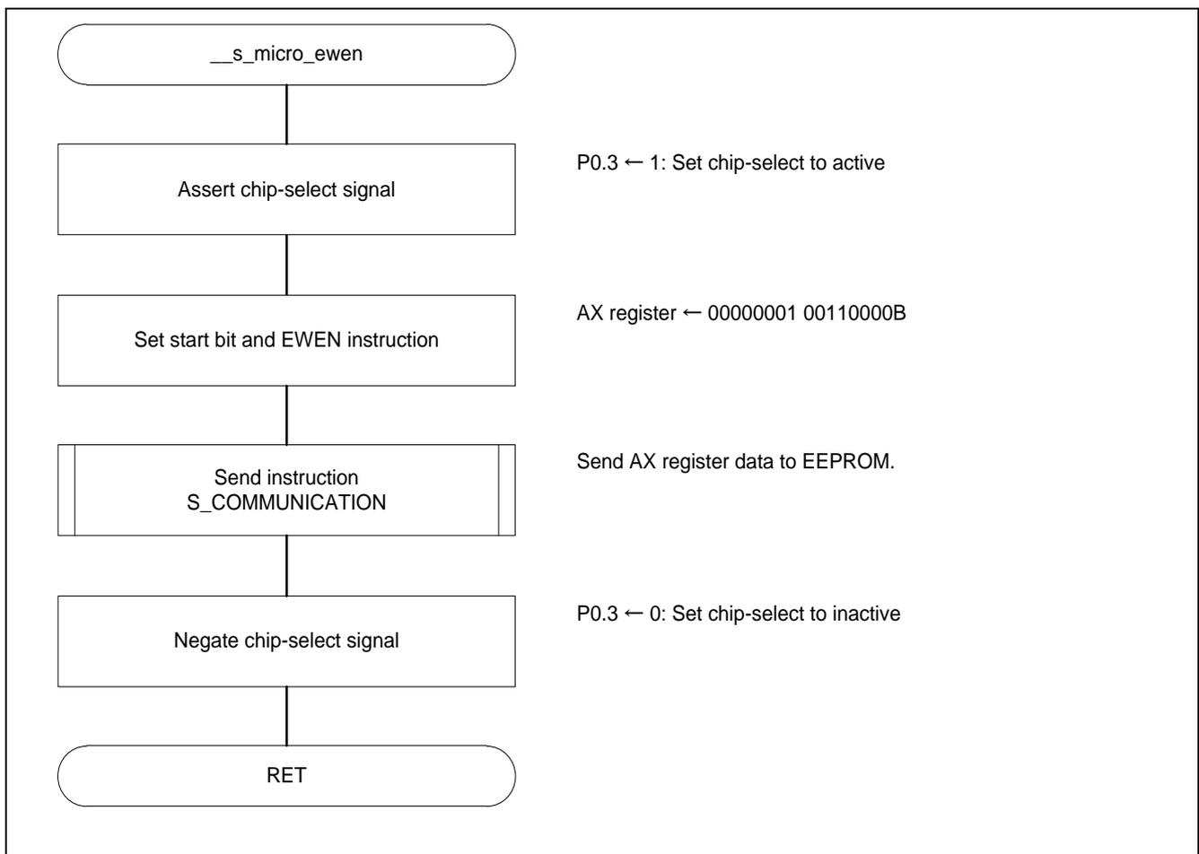
Figure 5.11 EEPROM Write Enabled Status Processing
