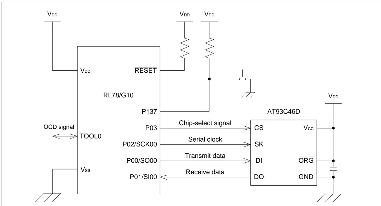
Figure 4.1 RL78/G10 and EEPROM (AT93C46D) Microwire Connection Example
