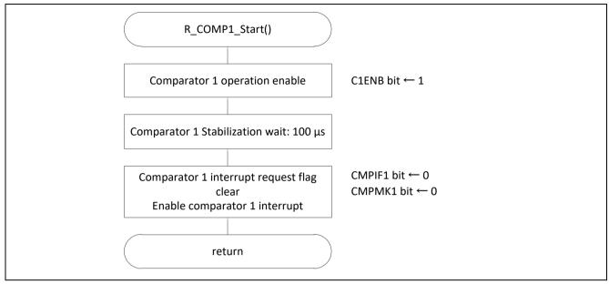
Figure 5.18 Starting Comparator 1 Operation
