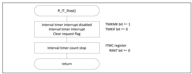
Figure 5.26 Stopping Interval Timer Operation
