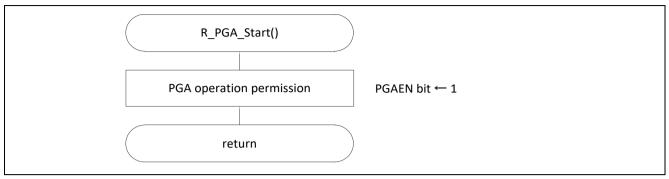
Figure 5.16 Starting PGA Operation
