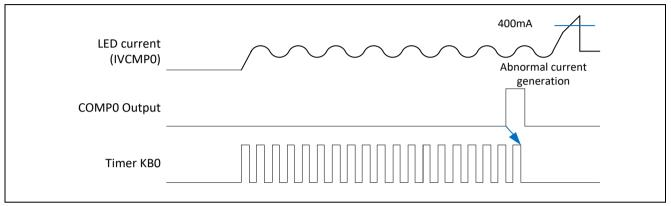
Figure 1.5 Forced Output Stop of Timer KB0
