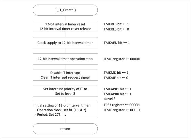
Figure 5.11 Setting 12-Bit Interval Timer
