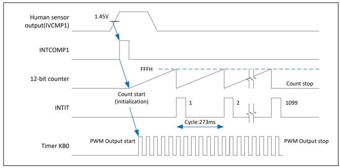
Figure 1.2 Detection of Human Sensor Output
