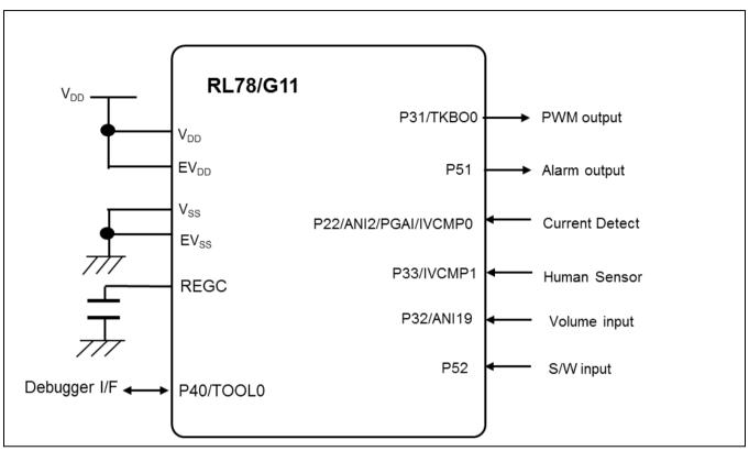
Figure 4.1 Hardware Configuration
