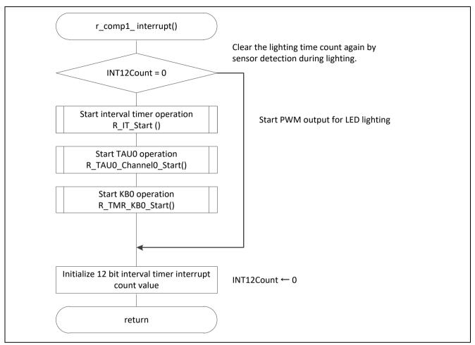
Figure 5.20 Comparator 1 Interrupt Operation
