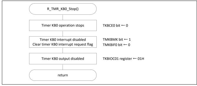
Figure 5.25 Stopping Timer KB0 Operation
