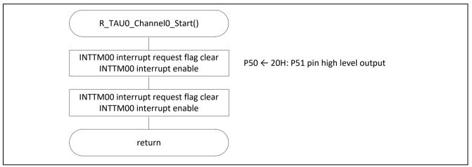
Figure 5.22 Starting Timer Array Unit Operation
