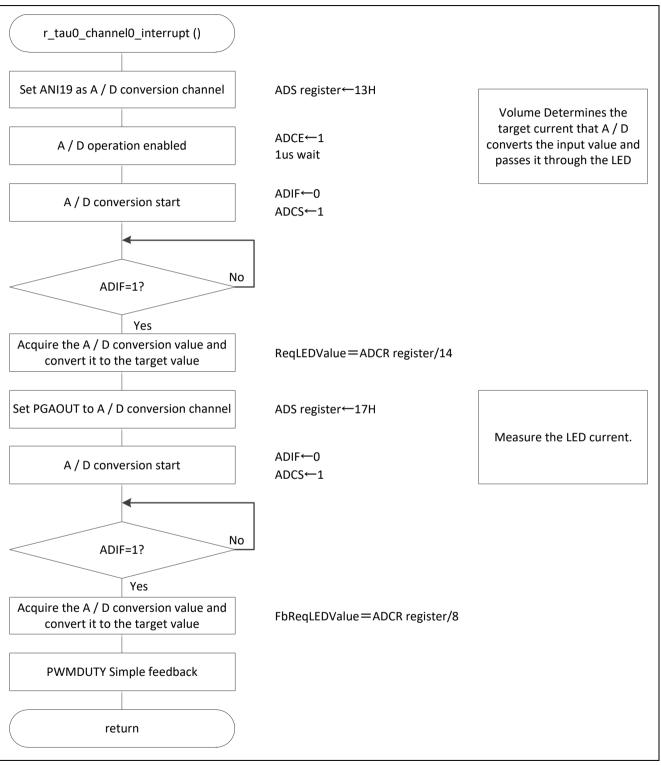
Figure 5.27 Timer Array Unit Interrupt Operation
