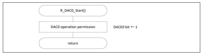
Figure 5.15 Starting D/A Converter Operation
