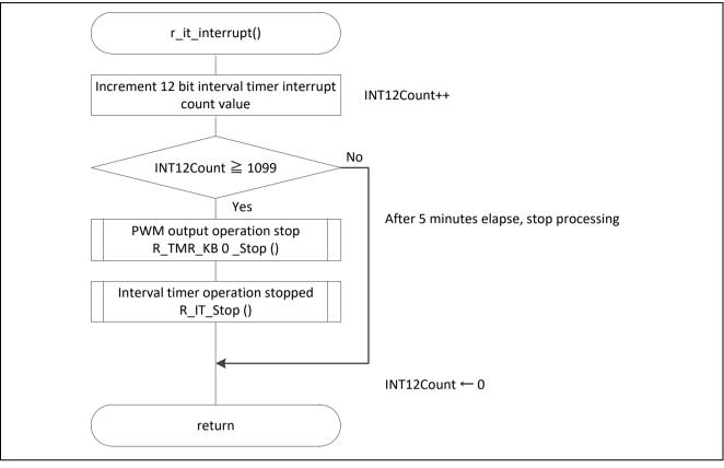
Figure 5.24 Starting Interval Timer Operation
