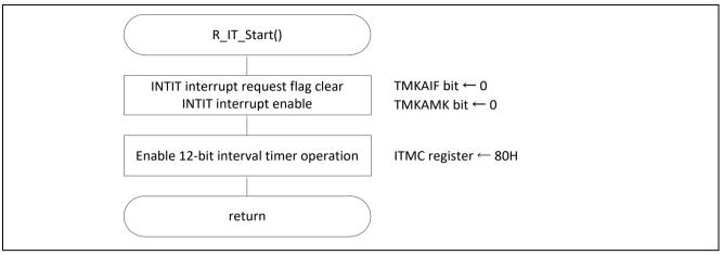
Figure 5.21 Starting Interval Timer Operation
