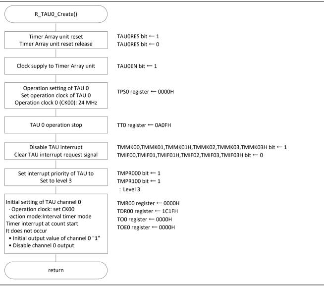
Figure 5.10 Setting Timer Array Unit
