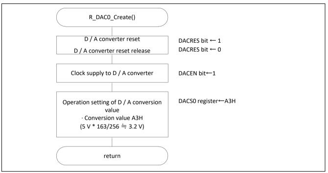
Figure 5.7 Setting D/A Converter
