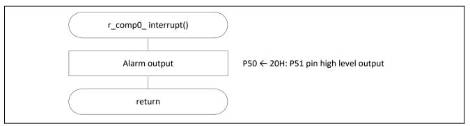
Figure 5.19 Comparator 0 Interrupt Operation
