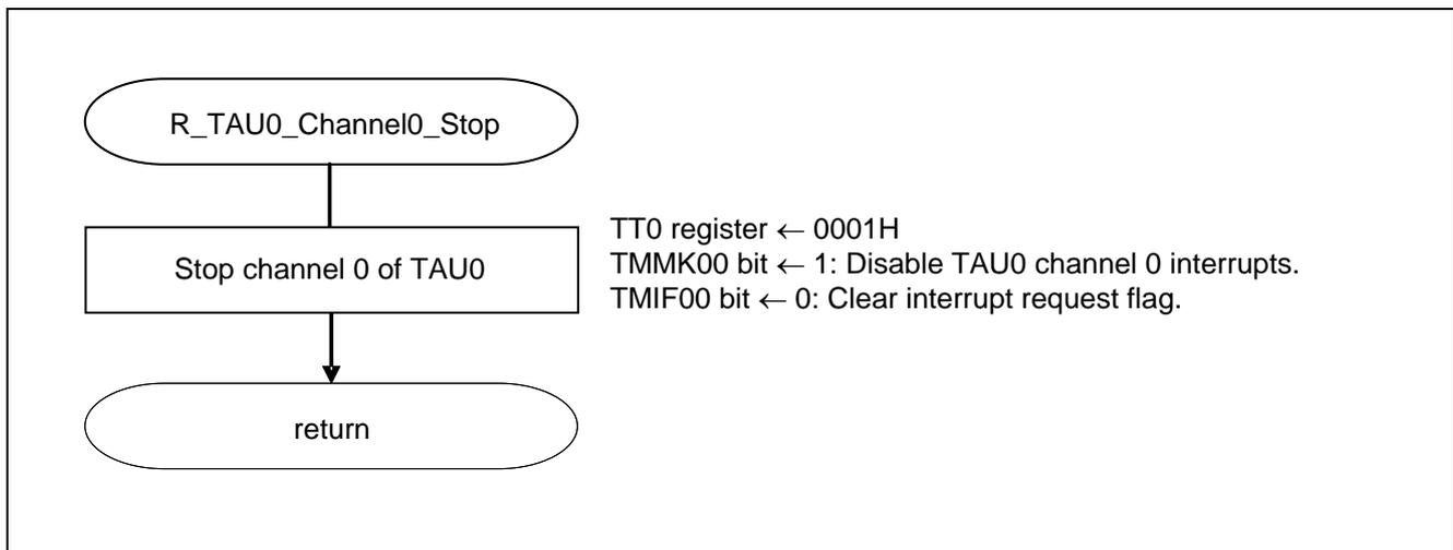
**Figure 5.24 Setting to Stop Channel 0 of TAU0**
