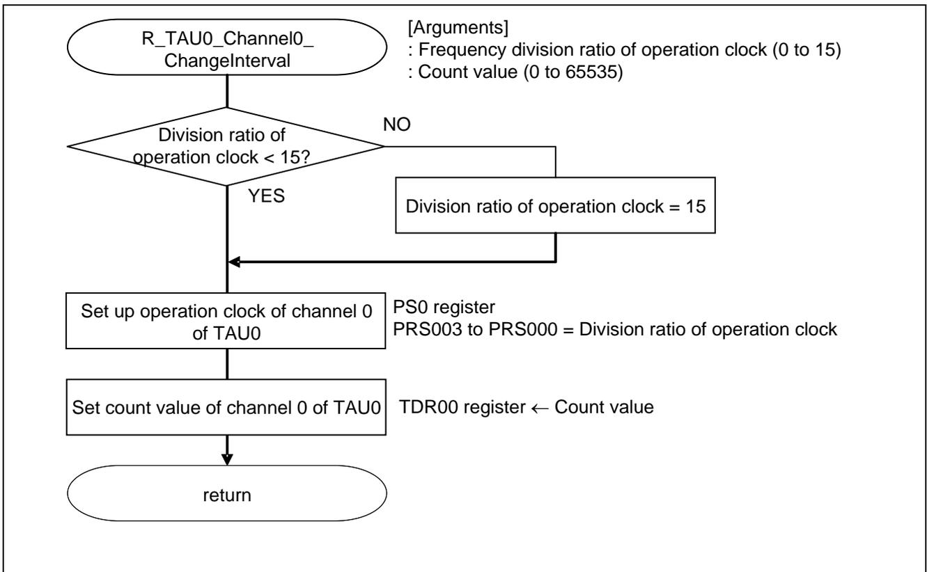
**Figure 5.23 Changing Interval of Channel 0 of TAU0**
