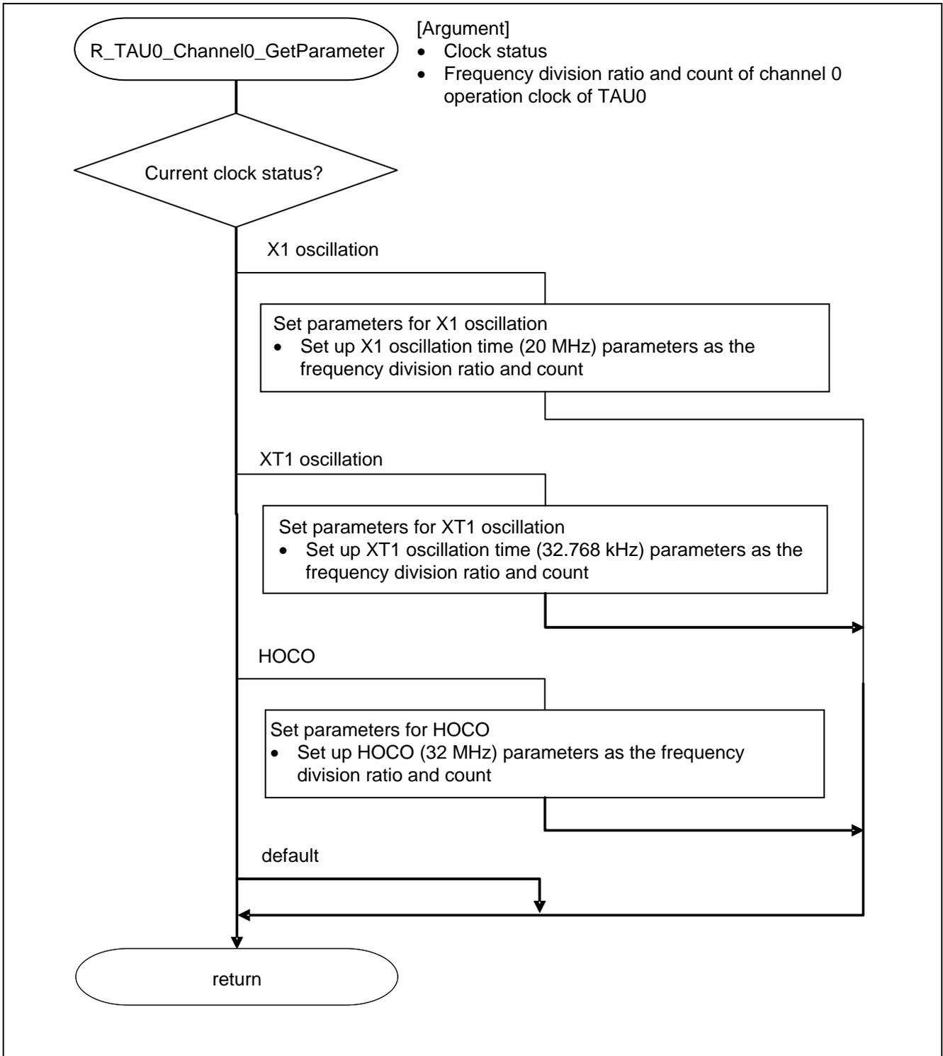
**Figure 5.21 Getting Parameters of Channel of TAU0**
