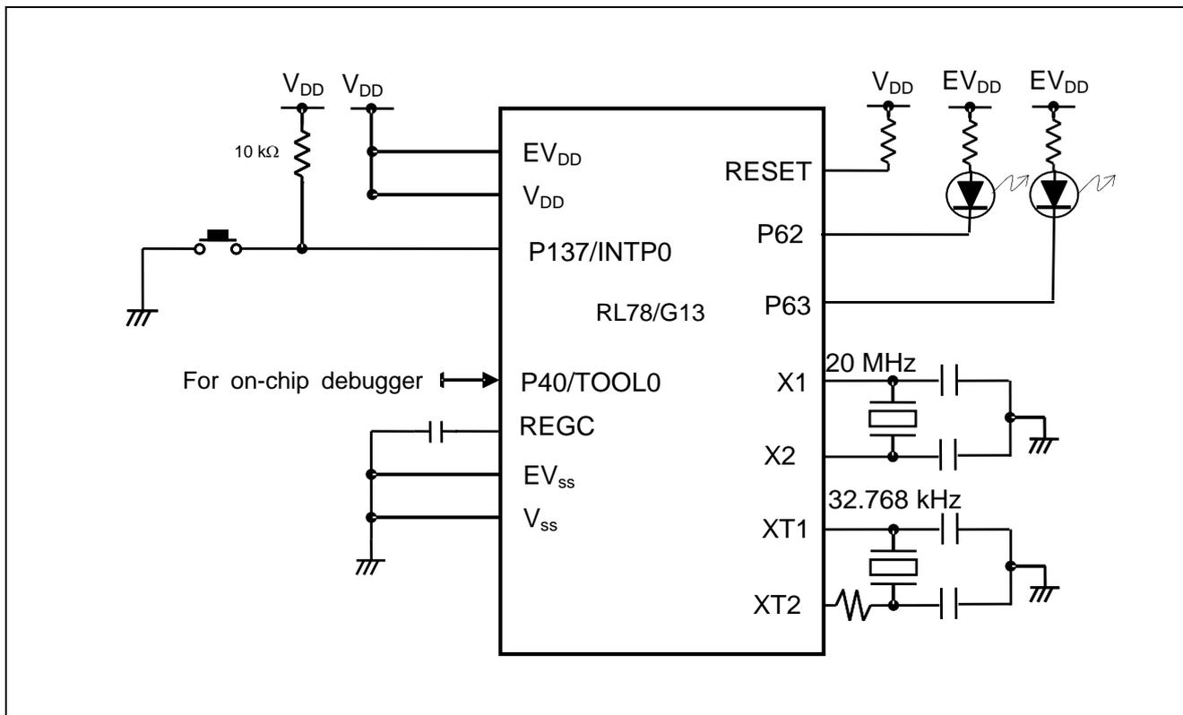
Figure 4.1 Hardware Configuration
