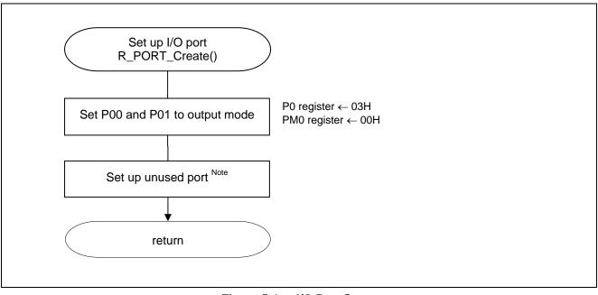
Figure 5.4 I/O Port Setup
