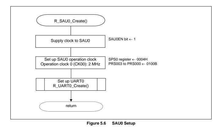
Caution: For details on the procedure for setting up the SAU0 (R\_SAU0\_Create ()), refer to the section entitled "Flowcharts" in RL78/G13 Serial Array Unit (UART Communication) Application Note (R01AN0459E).
