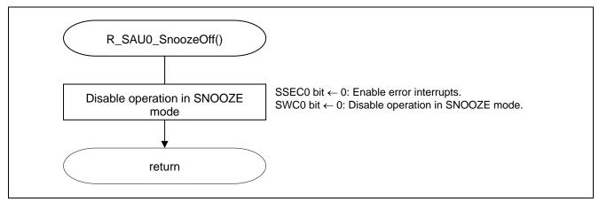
Figure 5.11 Disabling UART0 Operation in SNOOZE Mode
