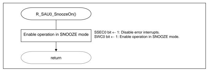
Figure 5.10 Enabling UART0 Operation in SNOOZE Mode
