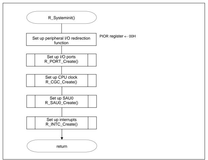
Figure 5.3 System Initialization Function
