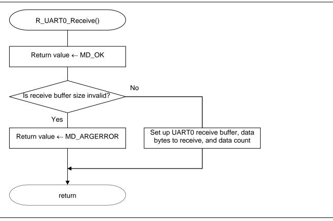
Figure 5.14 Setting up UART0 Receive Buffer
