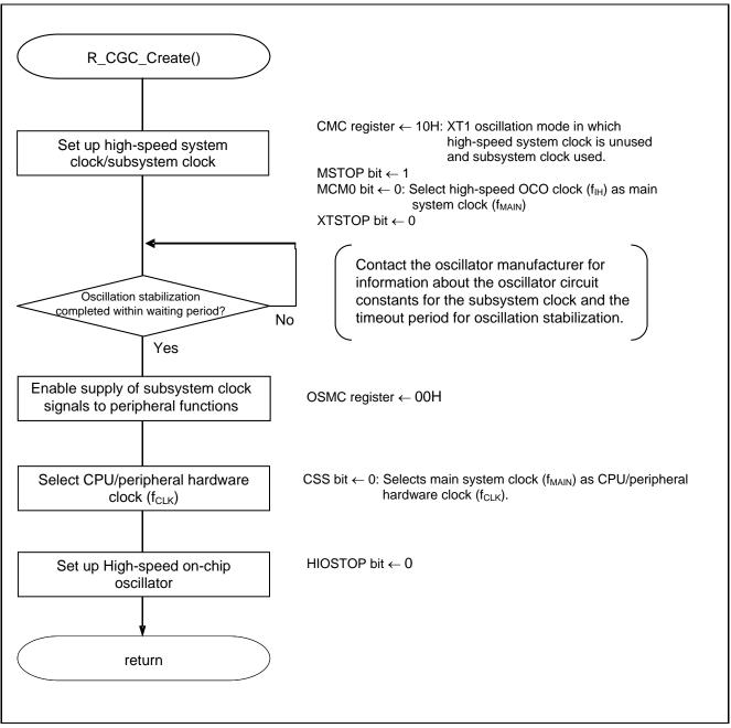
Figure 5.5 CPU Clock Setup
