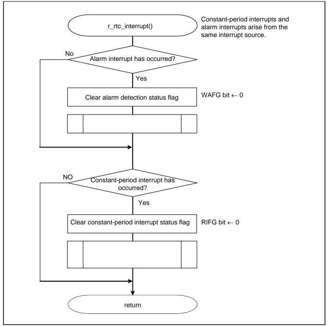
Figure 5.15 RTC Interrupt (INTRTC) Processing
