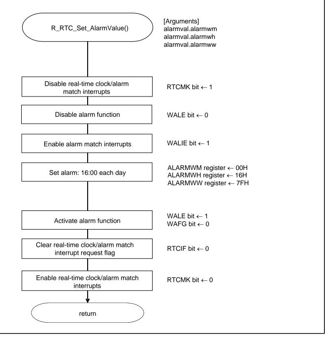
Figure 5.14 Alarm Generation Time Setup
