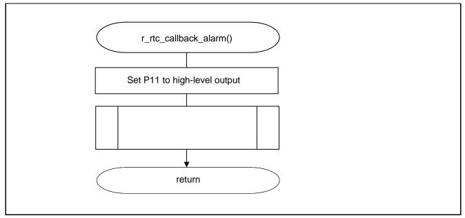
Figure 5.16 Alarm Interrupt Processing
