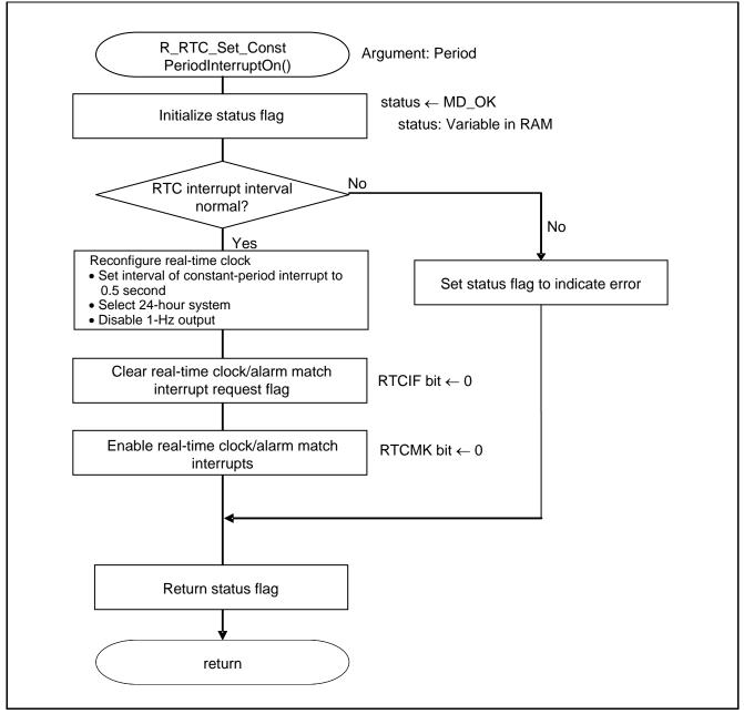
Figure 5.10 RTC Reconfiguration
