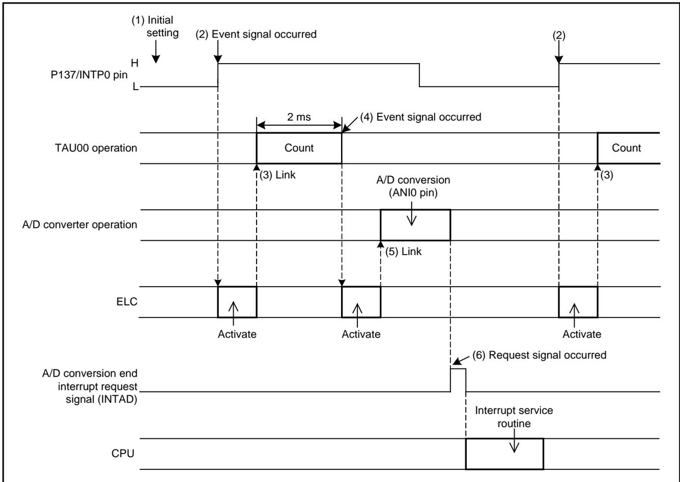
**Figure 5.1 Timing Diagram of the ELC and Peripheral Functions**
