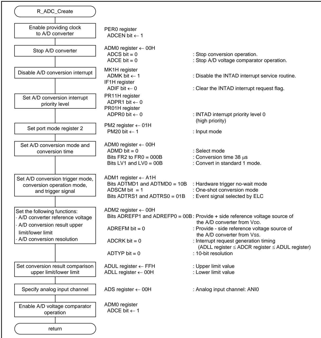
Figure 5.6 Initial Setting of the A/D Converter
