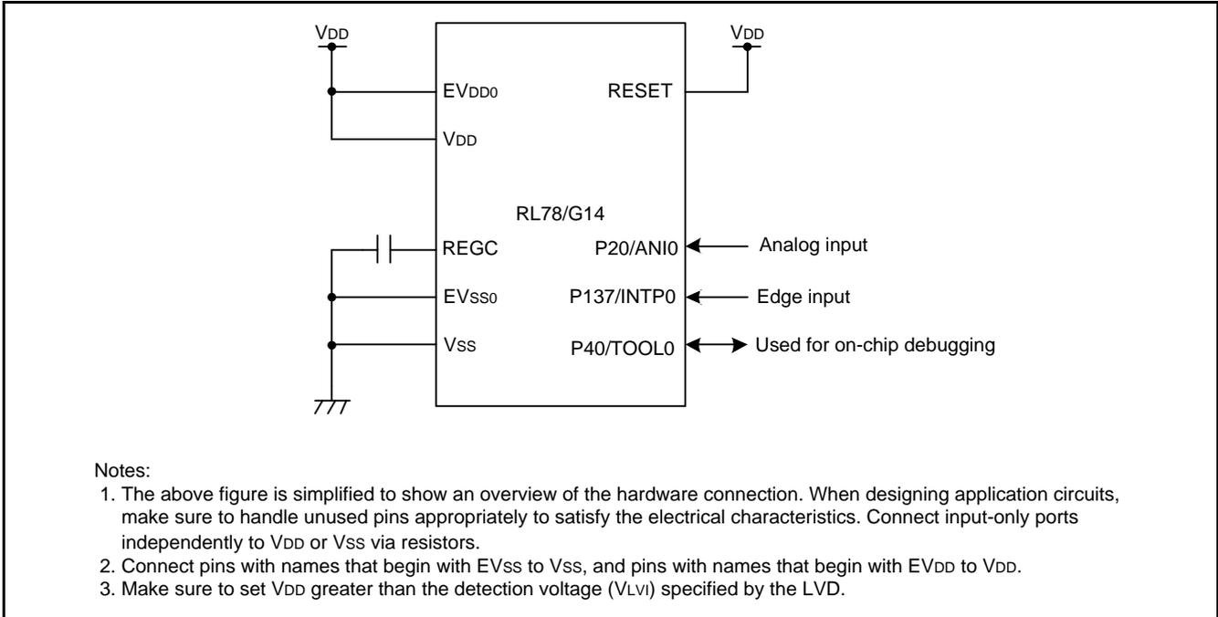
**Figure 4.1 Hardware Configuration**
