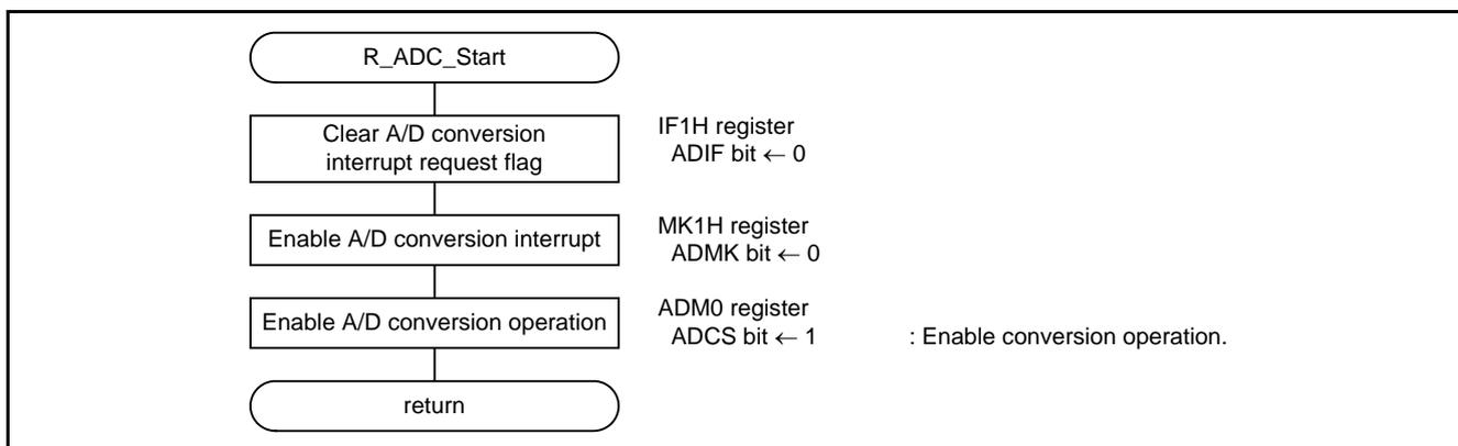
Figure 5.12 A/D Conversion Operation Enable Setting
