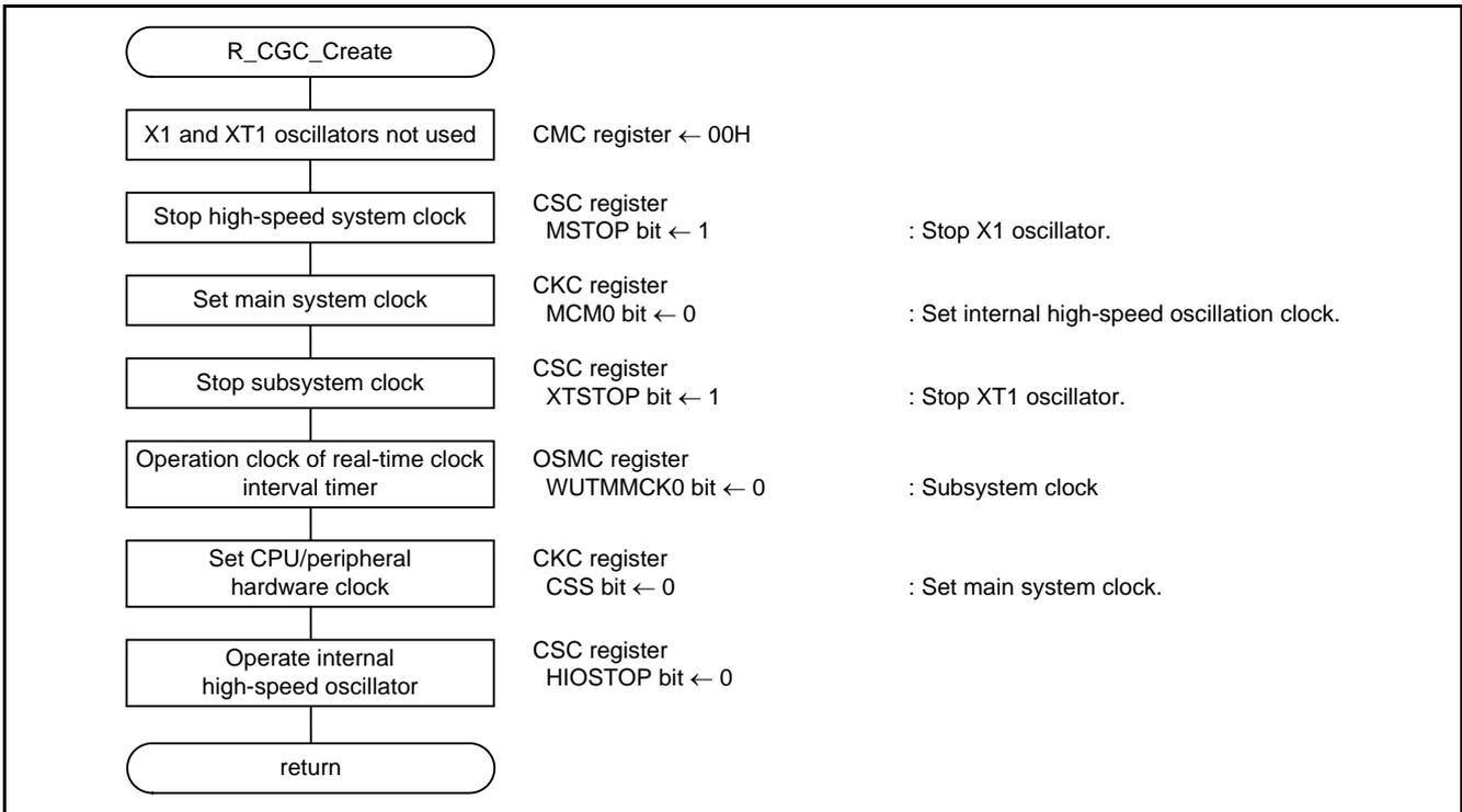
**Figure 5.5 Initial Setting of the CPU**
