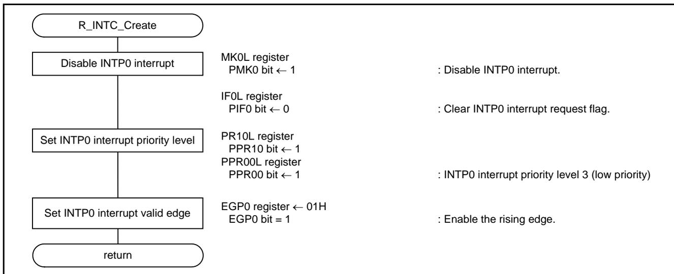
Figure 5.8 Initial Setting of INTPO
