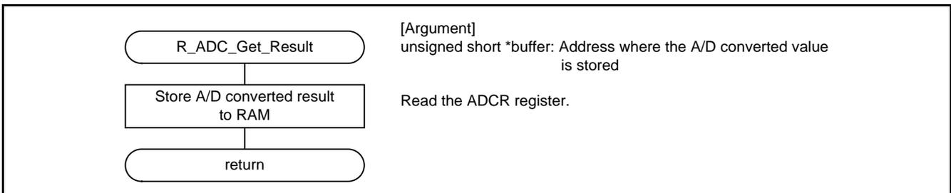
**Figure 5.14      A/D Converted Result Obtained**
