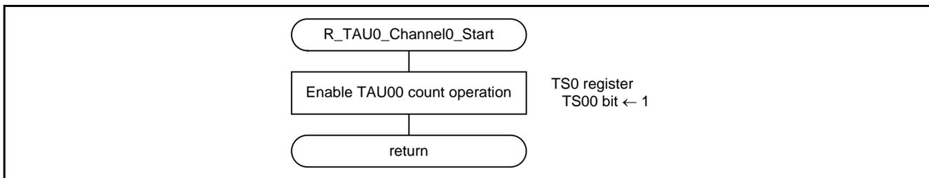
**Figure 5.11 TAU00 Operation Enable Setting**
