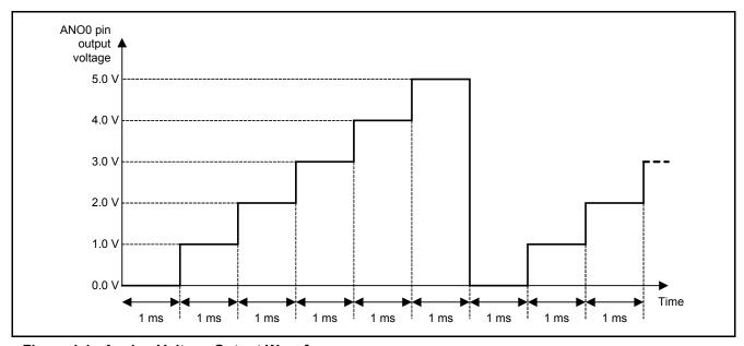
Figure 1.1 Analog Voltage Output Waveform
