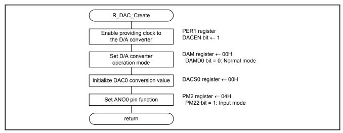
Figure 4.7 Initial Setting of the D/A Converter
