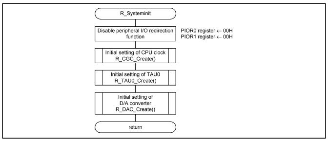
Figure 4.4 Initial Setting of Peripheral Functions
