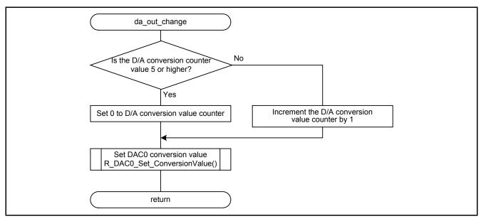
Figure 4.12 D/A Conversion Value Switch Processing
