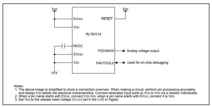
Figure 3.1 Hardware Configuration
