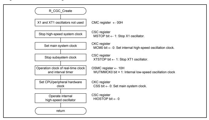
Figure 4.5 Initial Setting of the CPU Clock
