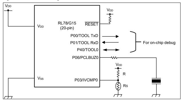
Note. This simplified circuit diagram was created to show an overview of connections only. When actually designing your circuit, make sure the design includes appropriate pin handling and meets electrical characteristic requirements (connect each input-only port to VDD or Vss through a resistor).
