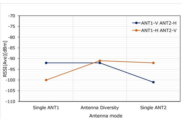
Figure 13. RSSI characteristics of Test 1
