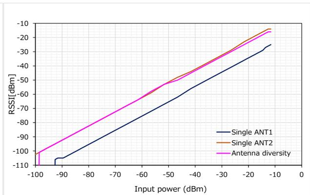
Figure 7. RSSI (ATT10dB on ANT1 side)
