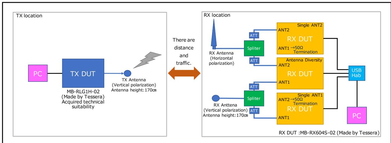
Figure 8. ANT1: Vertical polarization ANT2: Horizontal polarization
