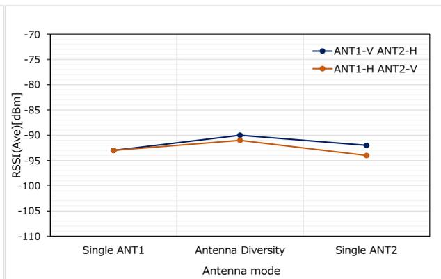
Figure 15. RSSI characteristics of Test 2
