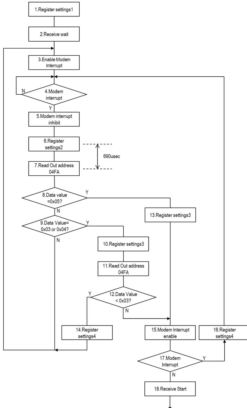
Figure 1. Flowchart for G1H/RAA604S00 based antenna diversity
