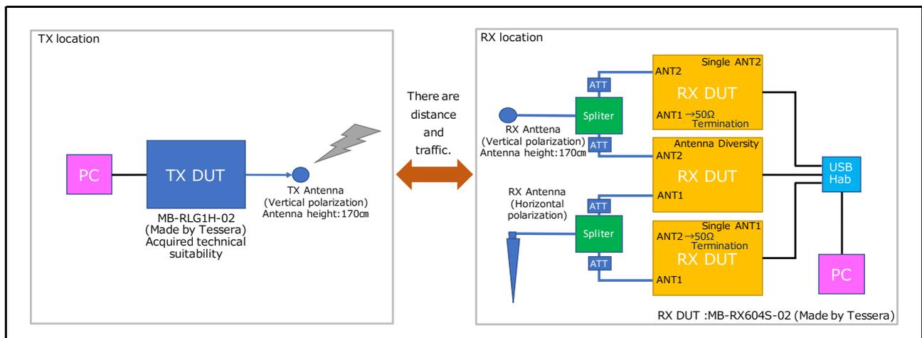
Figure 9. ANT1: Horizontal polarization ANT2: Vertical polarization
