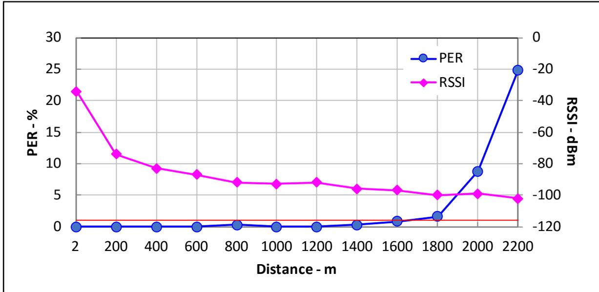
Figure 4-2 Packet error rate in each measurement point
