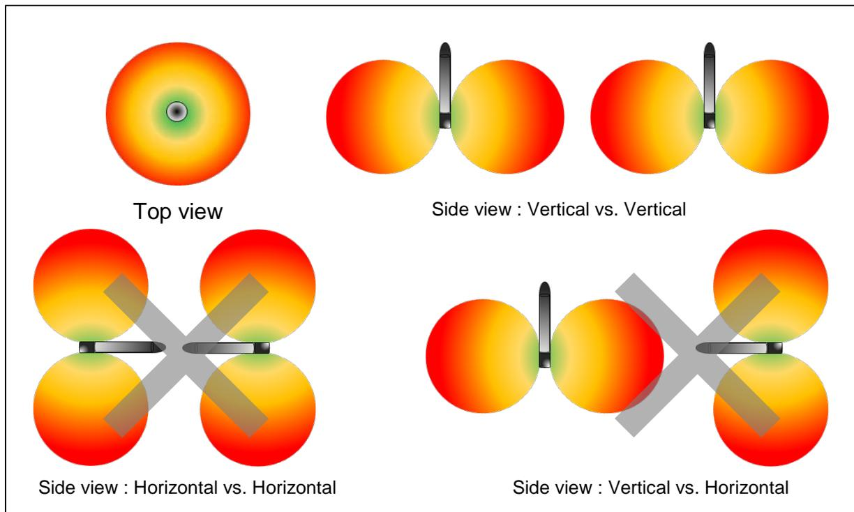
Figure 3-1 Radio field intensity and directivity of antenna
