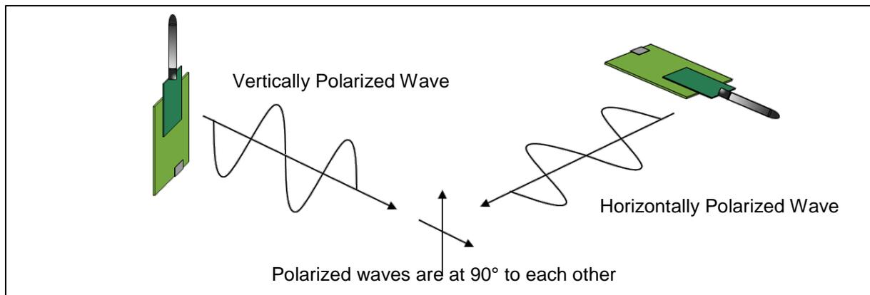
Figure 3-2 Antenna polarization
