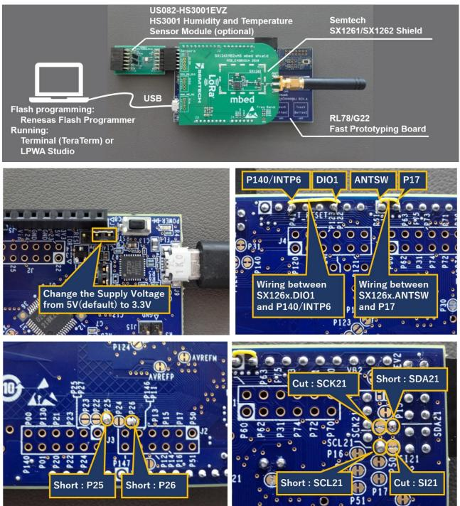
Note1: Power supply selection header (J17: default 5V) should be changed to 3.3V(J17 2-3 short).
