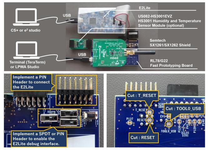
STEP1: Setup the board by referring to the basic setup section.
