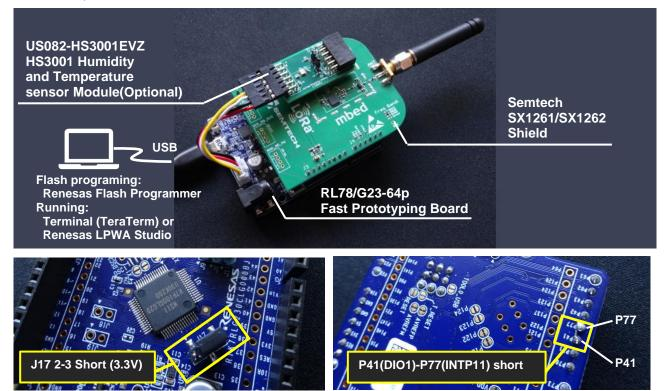
Note1: Power supply selection header (J17: default 5V) should be changed to 3.3V(J17 2-3 short).
