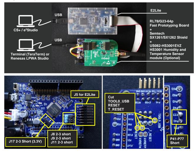
STEP1: Setup the board by referring to the basic setup section.
