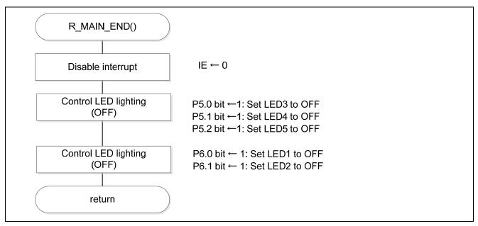
Figure 5.74 Status Transition End Processing
