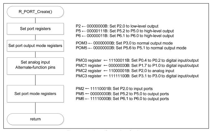
Figure 5.8 Input/Output Port Settings
