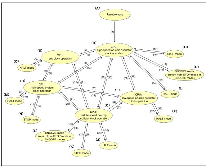
Figure 1.1 Operating Mode Status Transition Diagram
