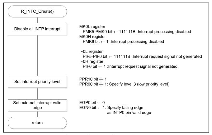
Figure 5.10 External Interrupt Setting
