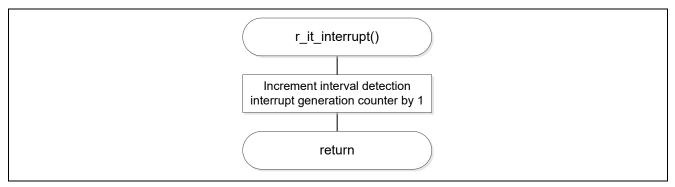
Figure 5.76 12-bit Interval Timer Interrupt Servicing
