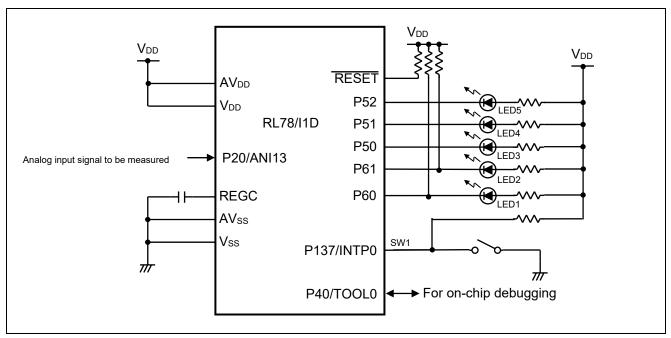
Figure 4.1 Hardware Configuration
