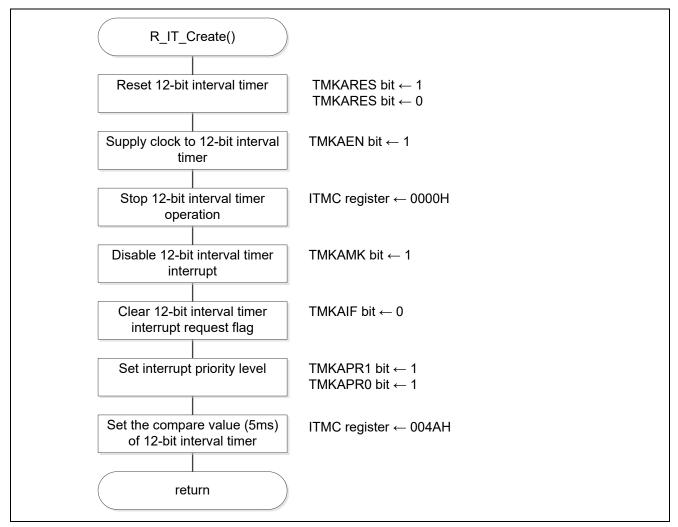
Figure 5.11 12-bit Interval Timer Setting
