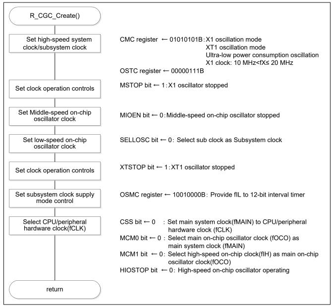
Figure 5.9 Clock Generator Setting
