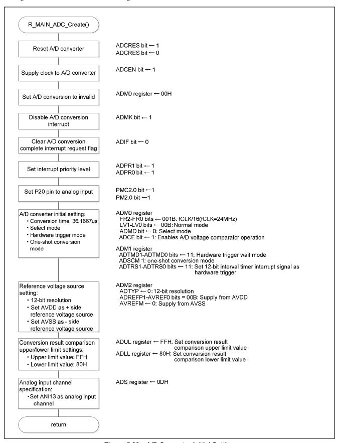
Figure 5.29 A/D Converter Initial Setting
