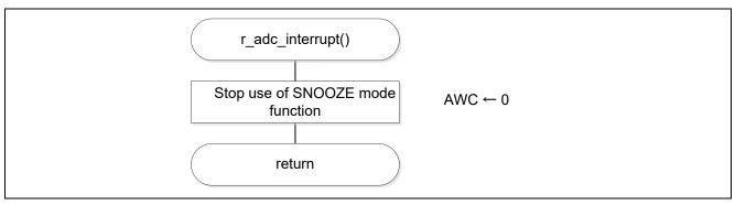
Figure 5.77 A/D Conversion Completion Interrupt Servicing
