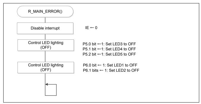
Figure 5.17 Error Processing of Status Transition
