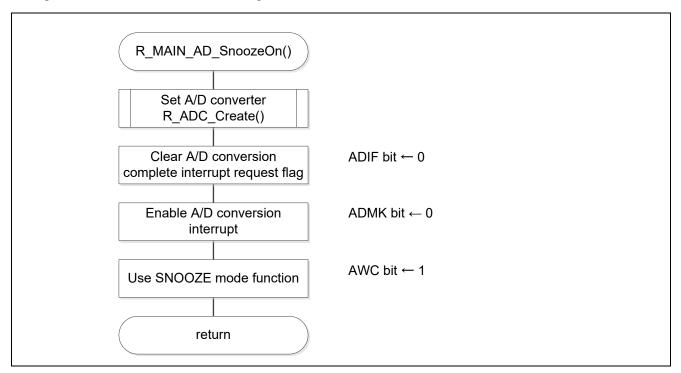
Figure 5.39 A/D Converter Setting
