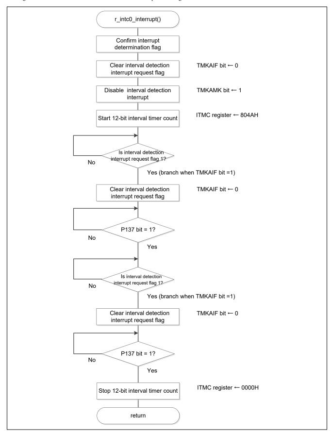
Figure 5.75 External Interrupt Servicing
