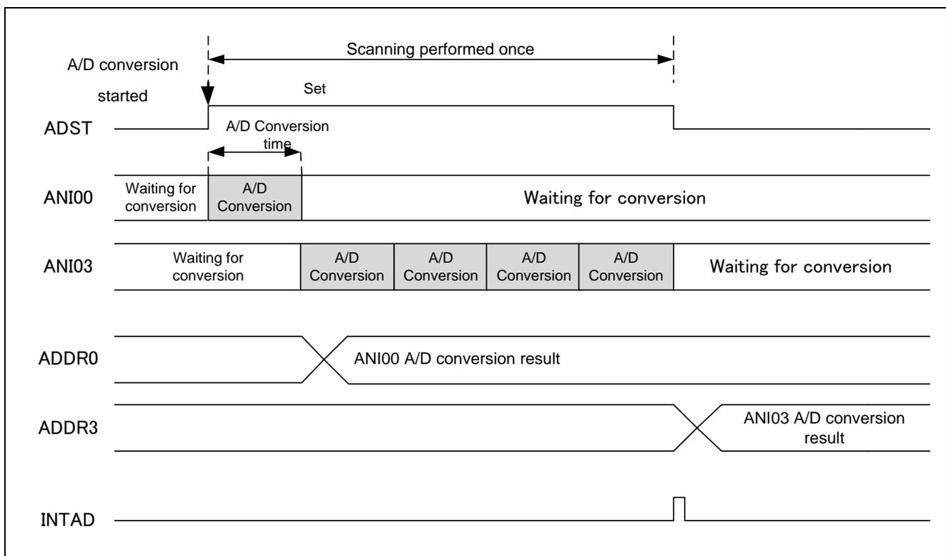
**Figure 1.1 Outline of the A/D Converter Conversion Processing**
