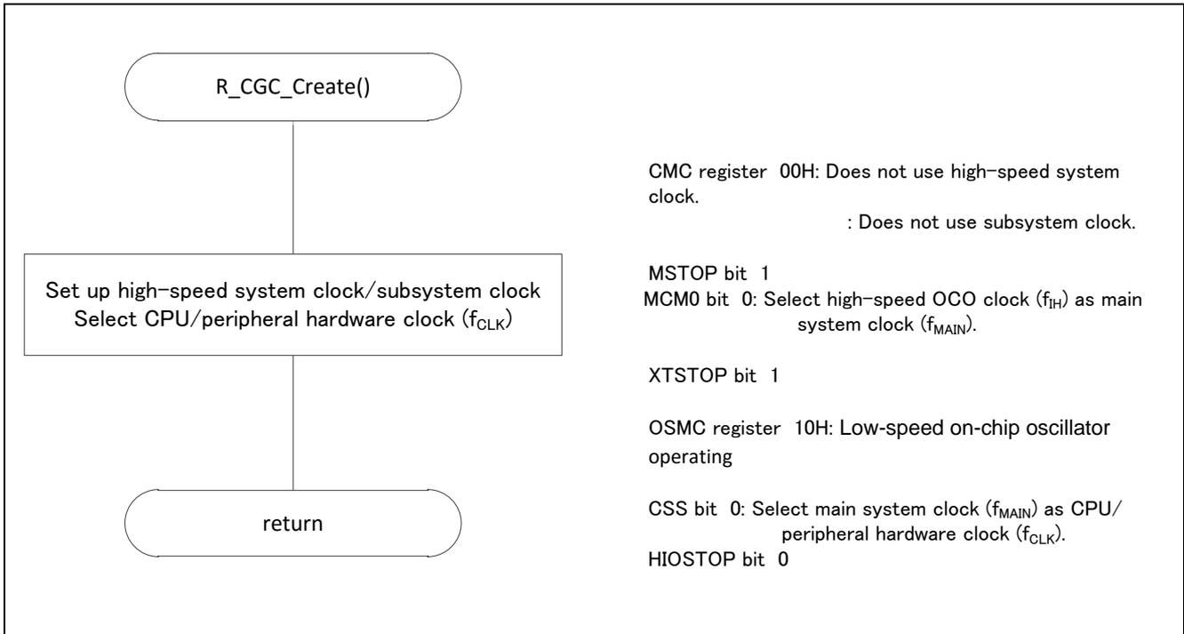
Figure 4.4 CPU Clock Setup
