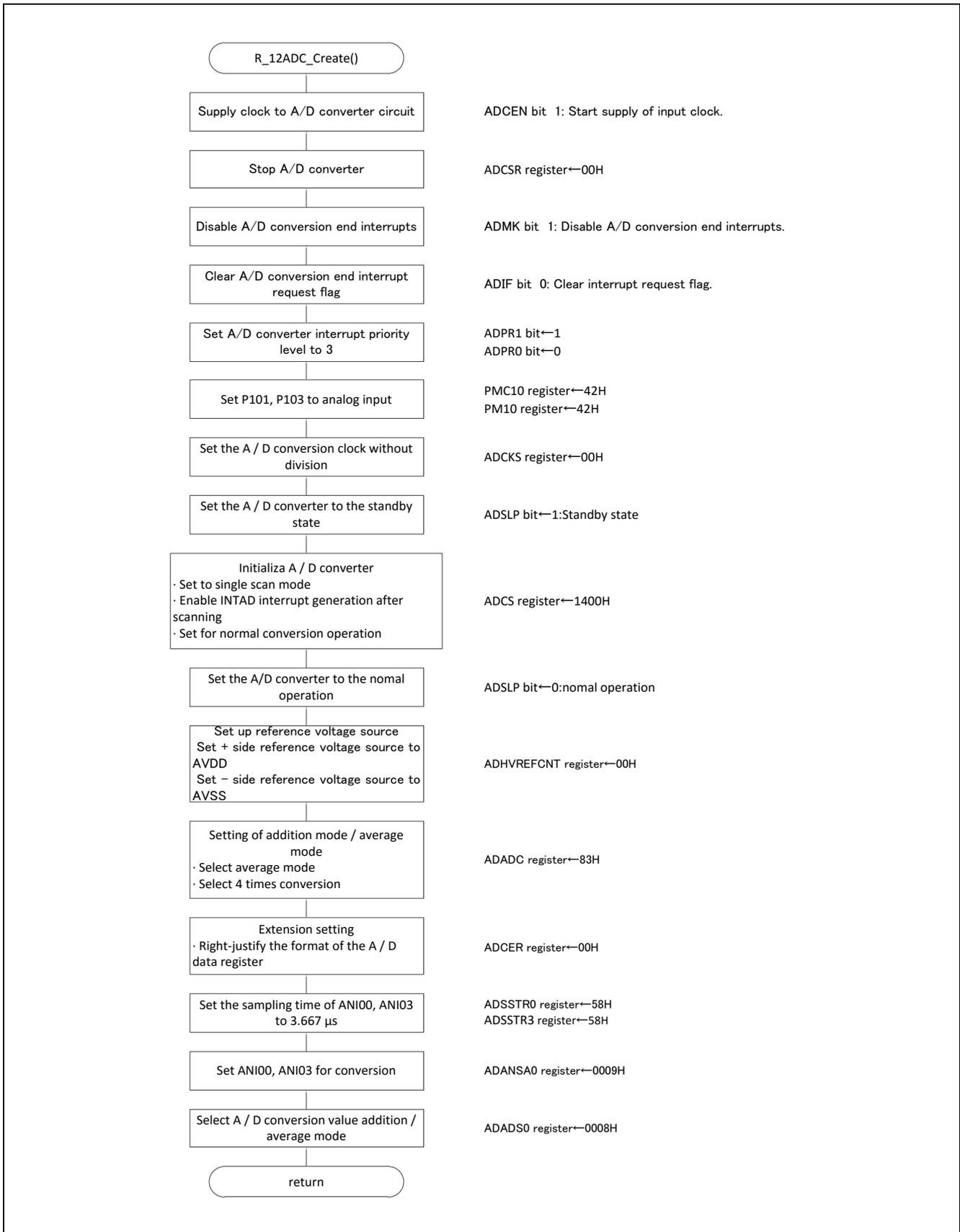
Figure 4.5 A/D Converter Setup
