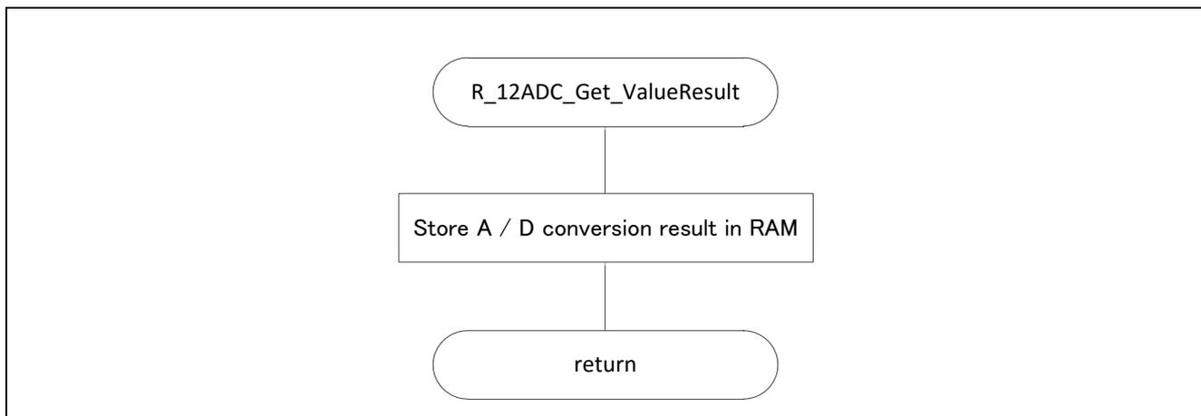
**Figure 4.9 Storing the A/D Conversion Results in RAM**
