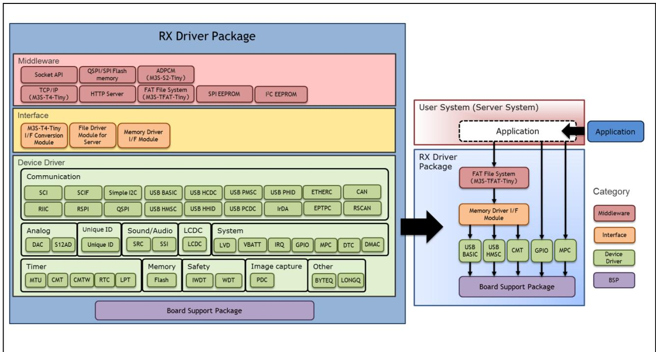
Figure 1-1 An Example of System Build
