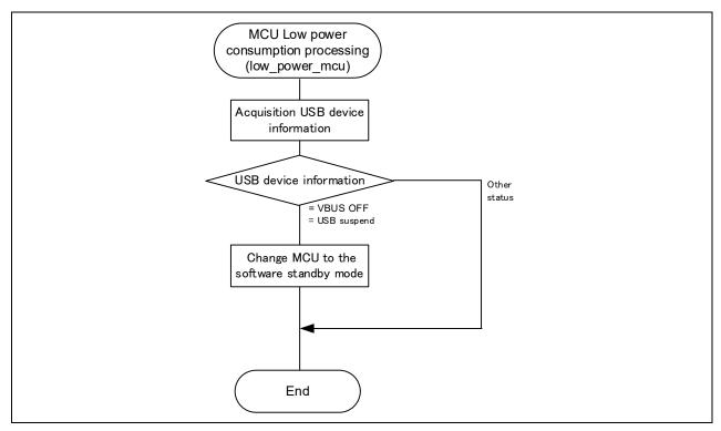
Figure 4-6 Flowchart of MCU Low Power Consumption Processing
