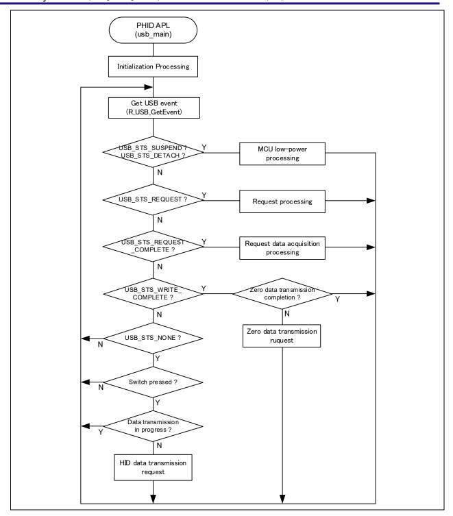
Figure 4-1 Main Loop Processing (Keyboard mode)
