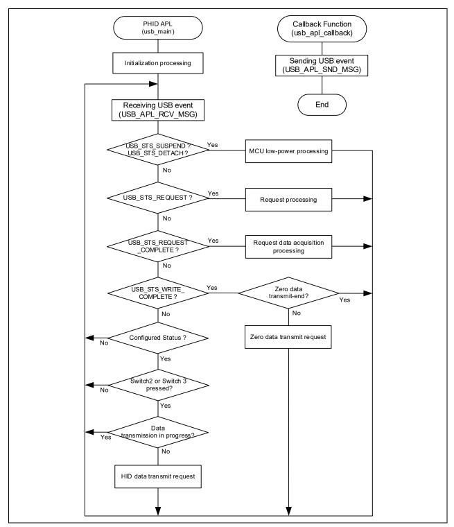
Figure 4-3 Main Loop Processing (Keyboard mode)
