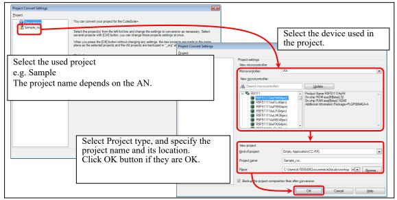
Figure 7-1 Using the e<sup>2</sup> studio project with CS+
