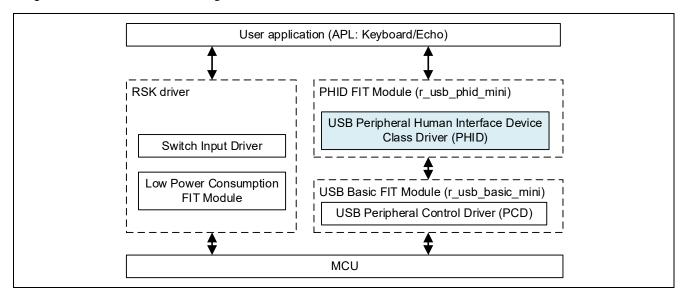
Figure 2-1 Module Configuration
