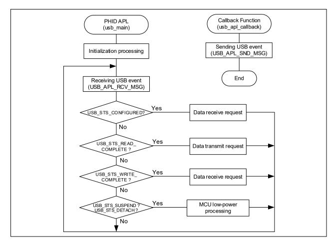
Figure 4-4 Main Loop Processing (Echo mode)
