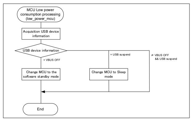
Figure 4-5 Flowchart of MCU Low Power Consumption Processing
