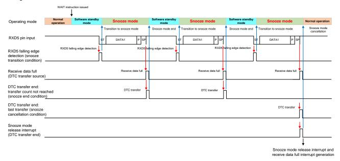
Figure 1.5 SCI Operation Example 3
