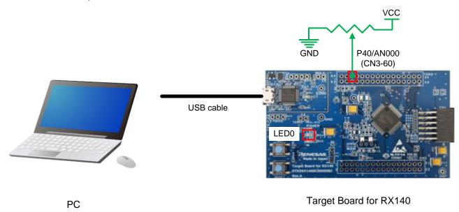
Figure 2.7 Target Board Connection Diagram
