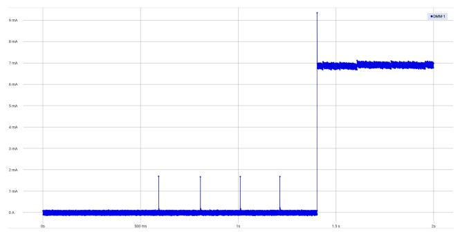
Figure 4.3 Current Value in Software Standby Mode and Snooze Mode (for SCI Operations)
