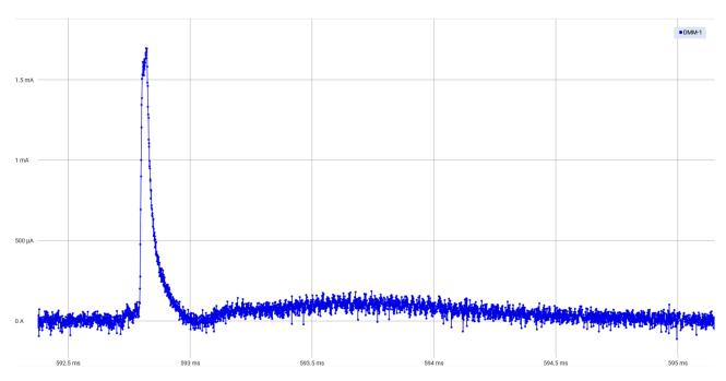
Figure 4.4 Current Value in Snooze Mode (for SCI Operations) (Magnified Image for the 1st Reception Operation)
