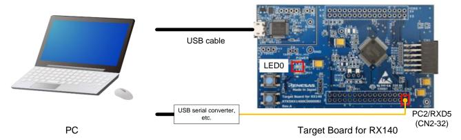
Figure 2.2 Target Board Connection Diagram
