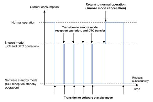
Figure 2.4 Illustration of Current Consumption during Reception Operation in SCI Asynchronous Mode
