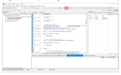
When the program runs, the indication of the status bar in the lower left corner of the window changes to **Standby**. After confirming that the status has changed to **Standby**, transmit serial data to the RXD5 pin.
