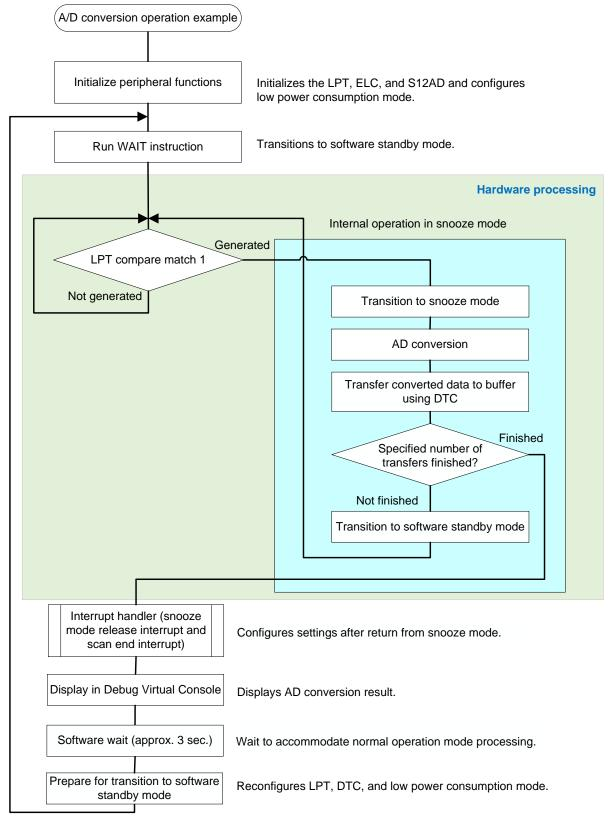
Figure 2.6 Outline Flowchart of Periodic A/D Conversion Operation Using LPT and S12AD
