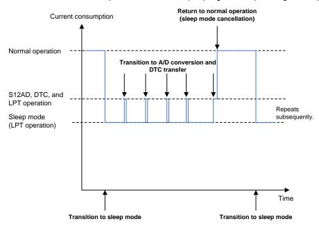
Figure 2.10 Illustration of Current Consumption during Periodic A/D Conversion Operation Using LPT and S12AD (Sleep Mode)
