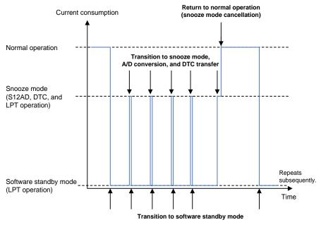
Figure 2.9 Illustration of Current Consumption during Periodic A/D Conversion Operation
