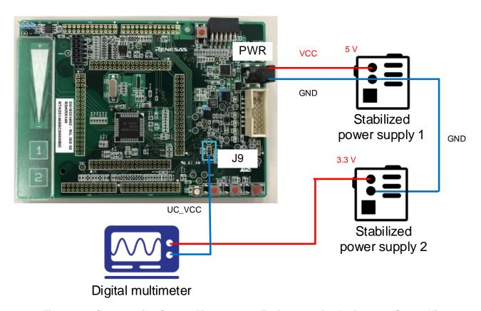
Figure 4.2 Consumption Current Measurement Environment for the Renesas Starter Kit
