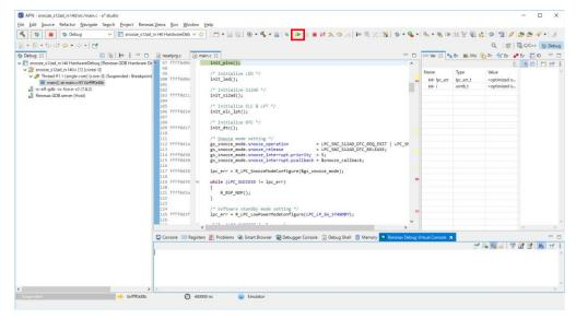
When the program runs, the indication of the status bar in the lower left corner of the window changes to **Standby**. After about five seconds, the status bar indication changes to **Running**, and five cycles' worth of A/D conversion results are displayed in the Renesas Debug Virtual Console.
