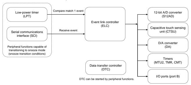
Figure 1.2 Peripheral Function Operation in Snooze Mode
