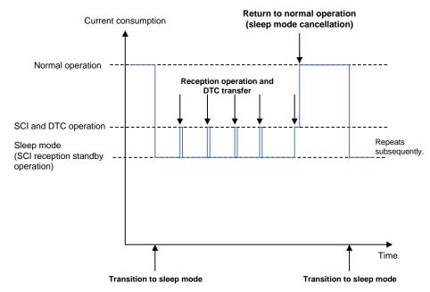
Figure 2.5 Illustration of Current Consumption during Reception Operation in SCI Asynchronous Mode (Sleep Mode)
