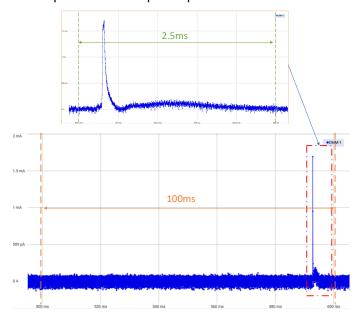
Figure 4.6 Example of Periodic Reception Operations by the SCI
