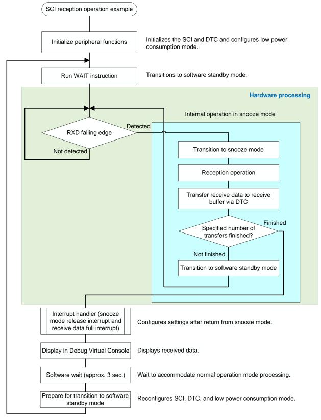
Figure 2.1 Outline Flowchart of Reception Operation in SCI Asynchronous Mode
