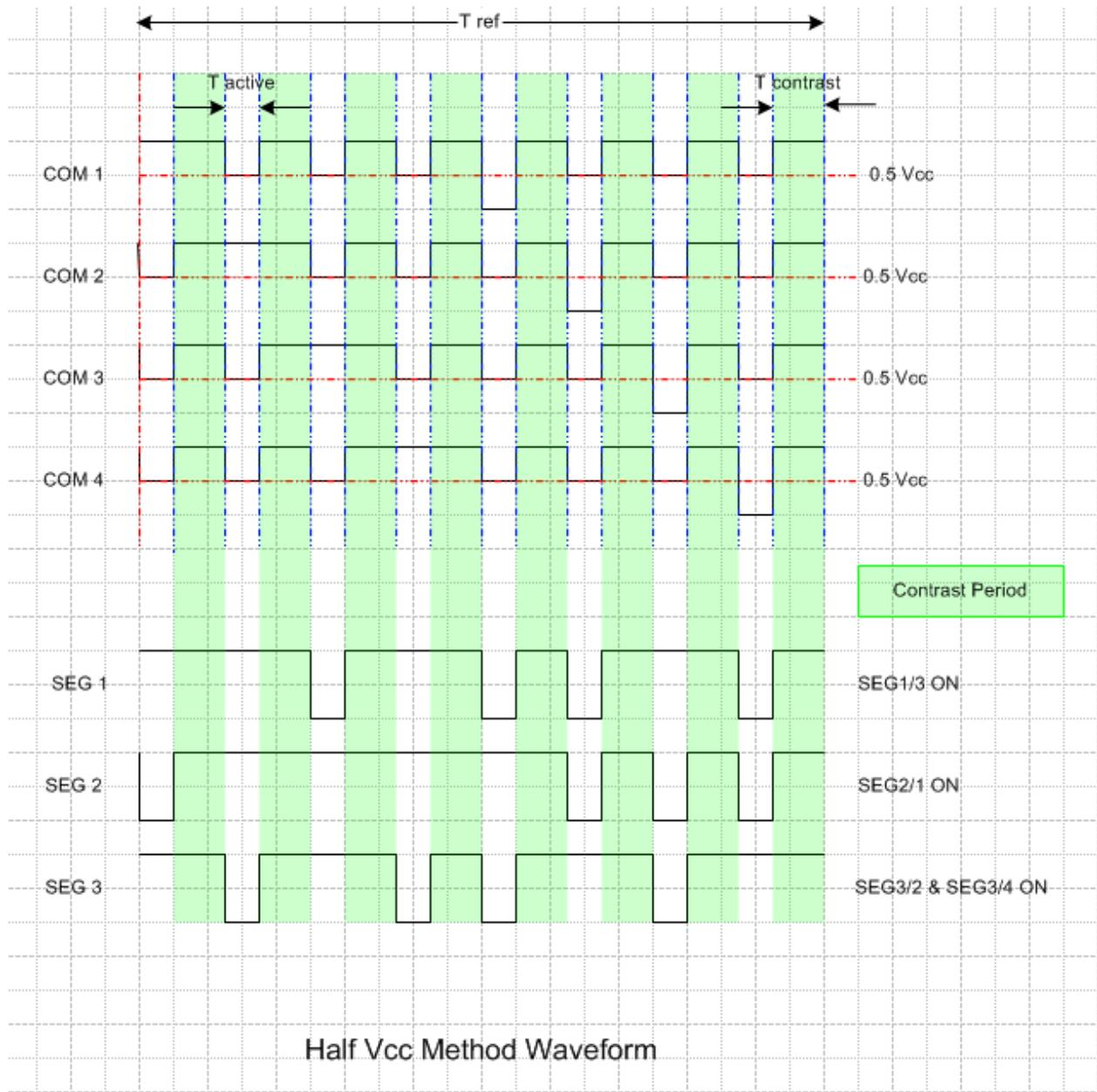
To examine the waveform on an oscilloscope, a trigger pulse has been added. This is available on TP2. A short pulse is generated everytime a new sequence of refresh has started. This is equivalent to the first state in the loop.
