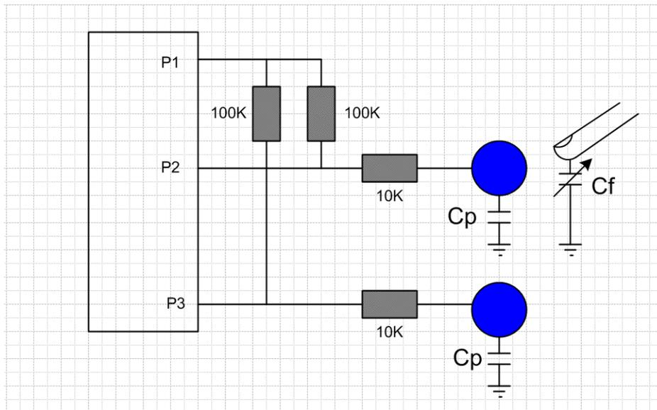
To increase the efficiency of this method, the user can also measure the fall time by setting P1 low. The fall time is shorter and therefore not as reliable as rise time. Preferably, it should not be used on its own but should be complimented with the rise time.
